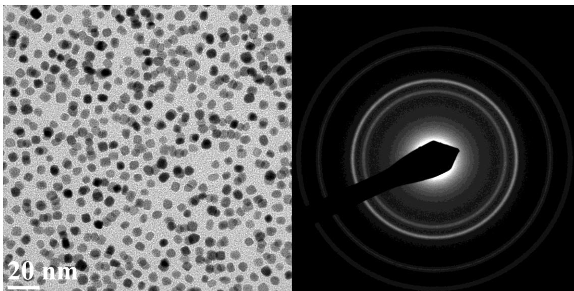
**Figure S-2.** Representative TEM image of 4.9 nm FePt nanoparticles.
