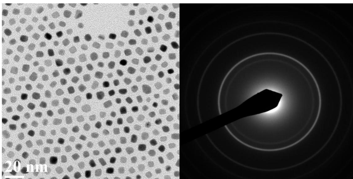
**Figure S-3.** Representative TEM image of 5.9 nm FePt nanoparticles.
