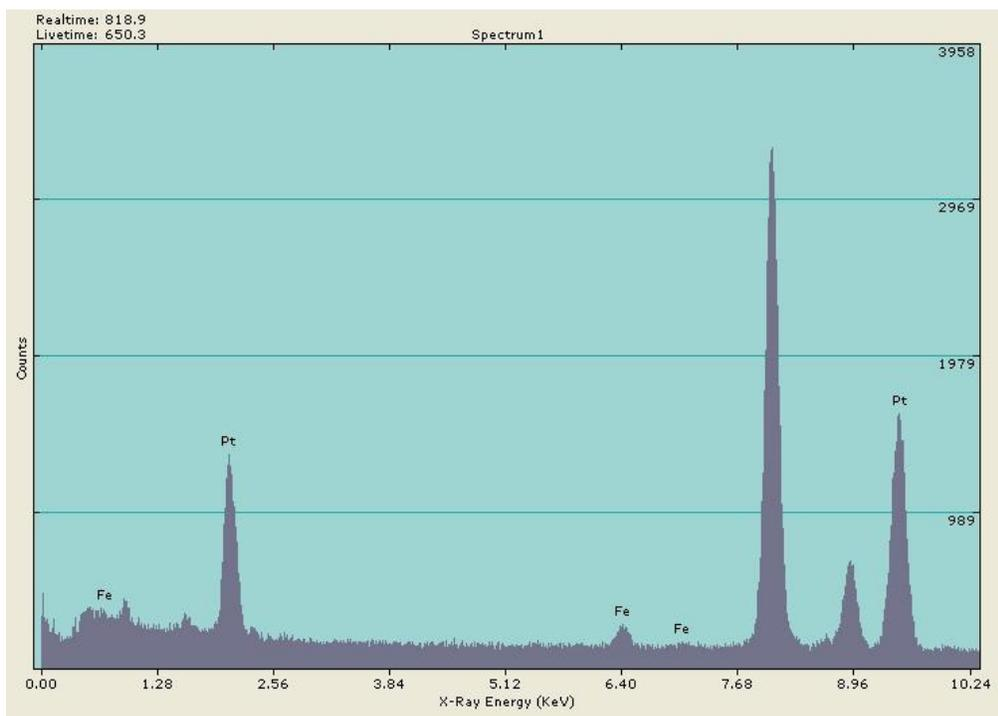
**Figure S-4.** EDS spectrum for 4.2 nm FePt nanoparticles.
