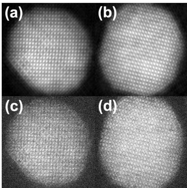
**Figure S-11.** (a-b) Filtered and (c-d) the original, unfiltered HAADF-STEM images showing the presence of the  $\text{FePt}_3$  phase forming on the edges of the nanoparticles.
