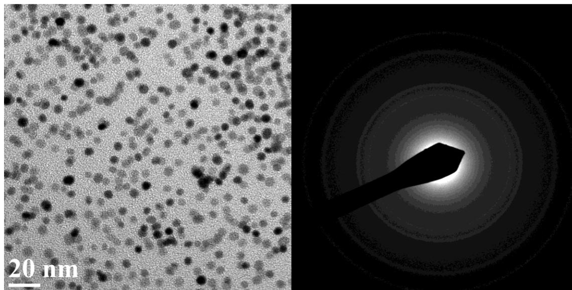
**Figure S-1.** Representative TEM image of 4.2 nm FePt nanoparticles.
