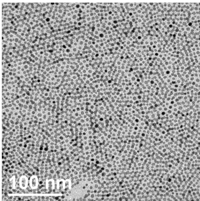
**Figure S-7.** TEM image of a spin cast array of a partial multilayer of 4.2 nm diameter FePt nanoparticles.
