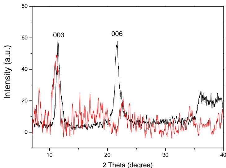
Figure S1. Wide-angle XRD patterns of As-synthesized Mg<sub>2</sub>Al-Cl-LDH nanoplates at room temperature (25 °C) and hydrothermally treated at 100 °C for 4 h (black) and the LDH@mSiO<sub>2</sub> core@shell NPs (red).
