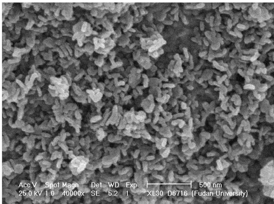
Figure S2. The SEM image of the as-synthesized core@shell nanocomposites LDH@mSiO<sub>2</sub> NPs.
