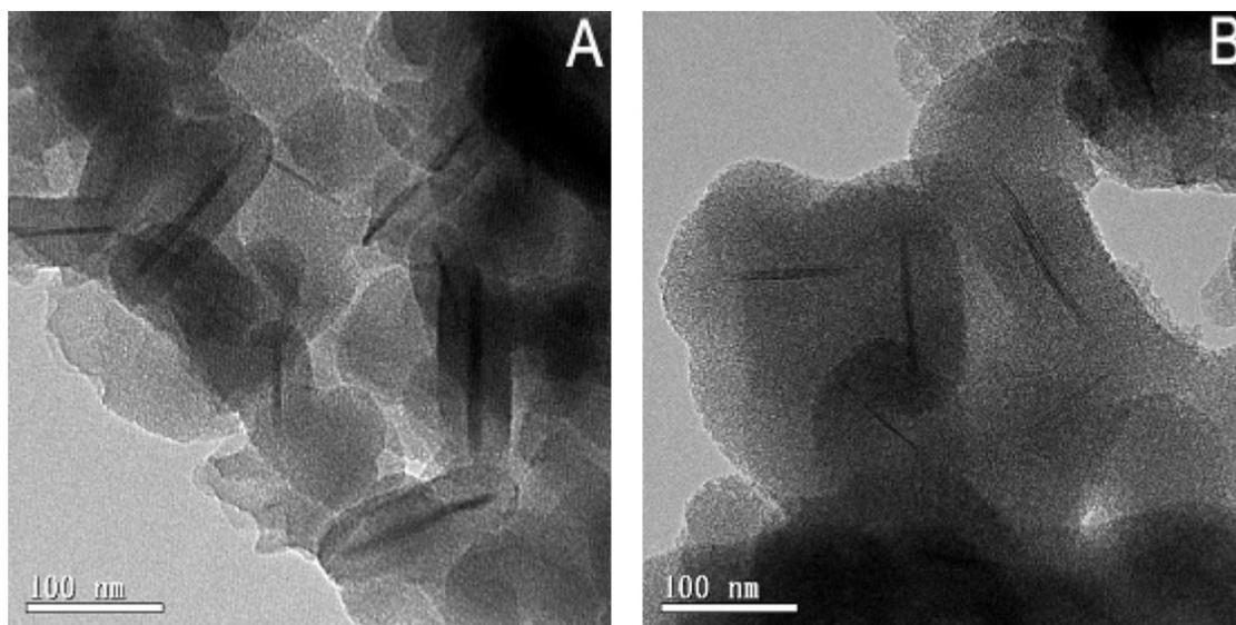
Figure S3. TEM images of the core@shell nanocomposites LDH@mSiO<sub>2</sub> NPs with a thickness of 20 nm (A) and 50 nm (B).
