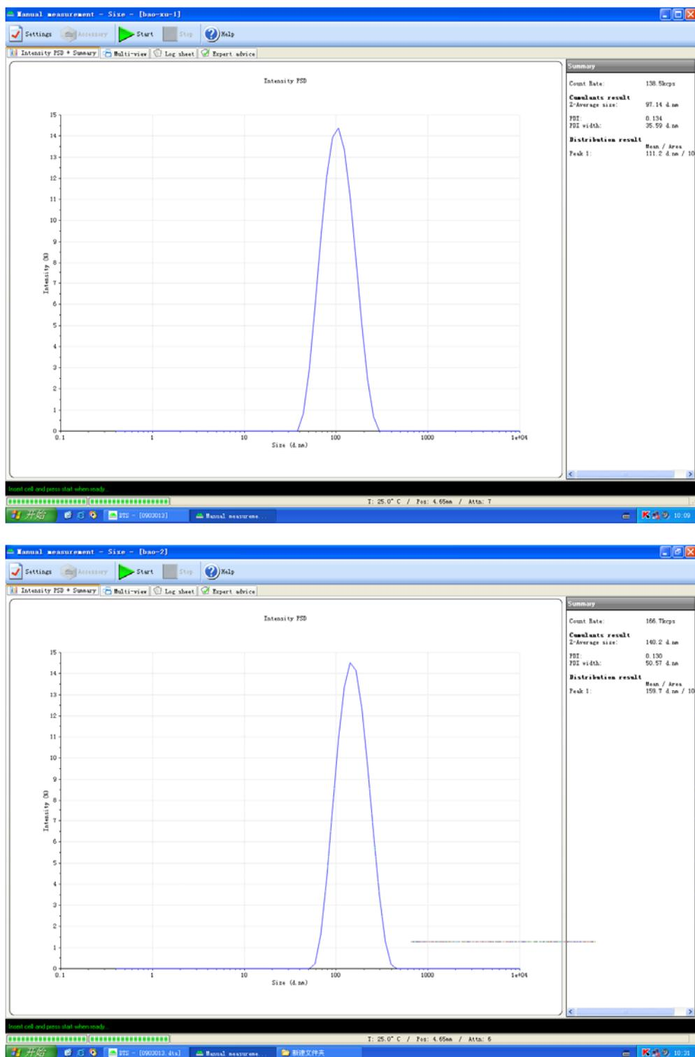
Figure S4. Hydrodynamic diameter distributions of LDH NPs (up) and LDH@mSiO<sub>2</sub> NPs with a thickness of 20 nm (down).
