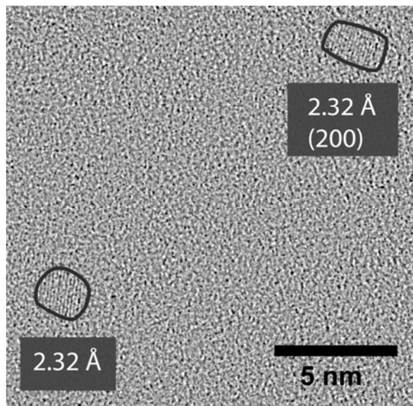
Fig. 3s TEM image of an ultramicrotome cut of polyHEMA based nanocomposite with 20wt%  $\text{MgF}_2$ .
