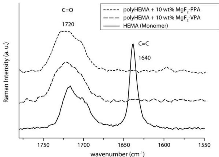
Fig. 1s Raman spectra of composites consisting of PPA and VPA modified magnesium fluoride nanoparticles in polyHEMA.
