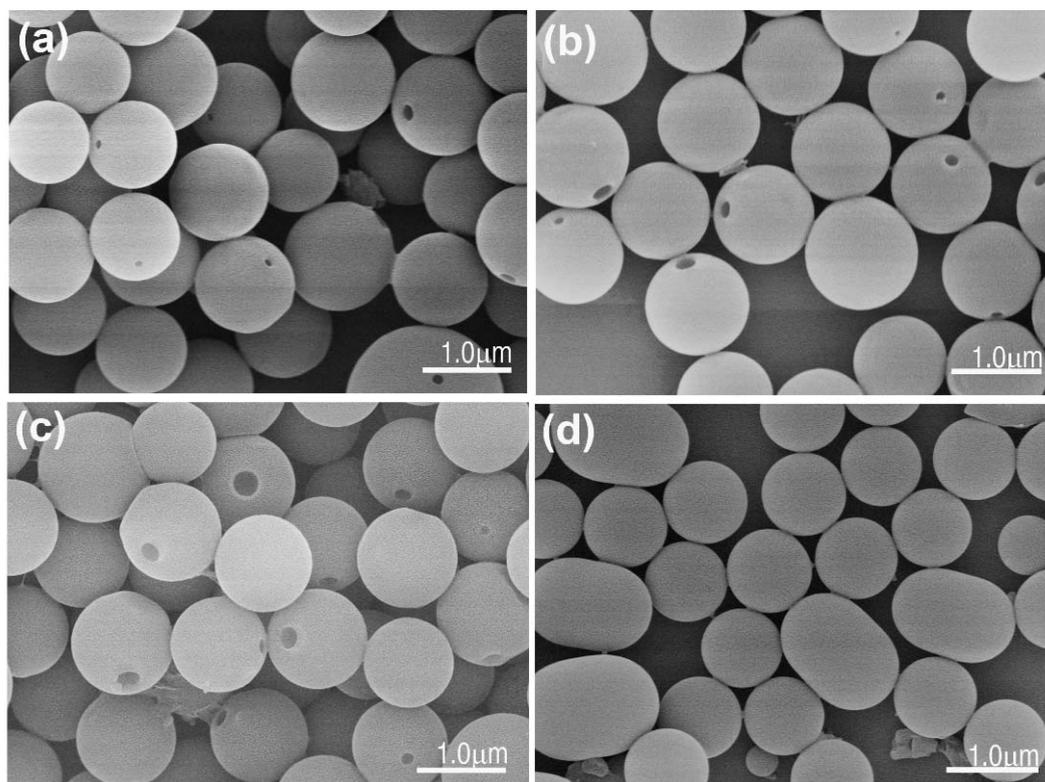
**Fig. S3.** SEM images of the obtained polystyrene microspheres when different amounts of monomer (styrene) are added: (a) 1.5 mL, (b) 2.0 mL, (c) 2.5 mL, (d) 4.0 mL. Insufficiency of monomer leads to broad size distribution, while an excessive monomer results in coalescence.
