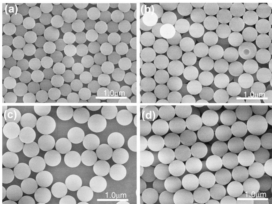
**Fig. S5.** SEM images of polystyrene microspheres prepared by conventional polymerization with reaction conditions of 0.5 mg/mL of AIBN, 55 mg/mL of St, and 5.0 mg/mL of PVP, at different heating time: (a) 30 min, (b) 60 min, (c) 120 min, and (d) 180 min. As revealed by the SEM images, through the conventional method, polymer spheres grow slower (~400 nm at 30 min, and ~530 nm at 180 min), and almost all the products are solid spheres without pores.
