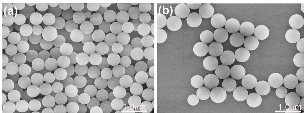
**Fig. S1.** SEM images of polystyrene microspheres obtained after irradiation of microwave for (a) 40 min and (b) 60 min at AIBN concentration of 0.125 mg/mL. As polymerization goes on, the spheres grow larger ((a): ~480 nm, (b): ~570 nm)), but no pore comes into being.
