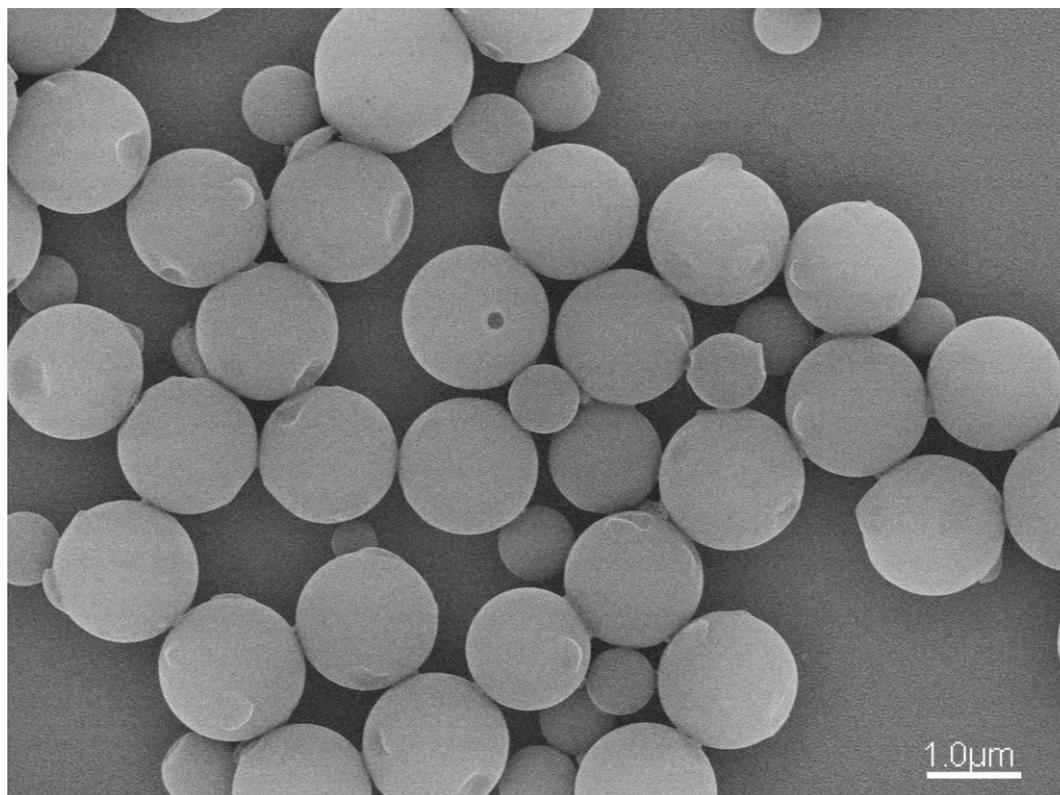
**Fig. S2.** SEM image of polystyrene microspheres obtained when the microwave-assisted polymerization is conducted for 60 min. From the SEM image, it is found that the surfaces of the spheres are not smooth, and at the same time some small spheres are also observed.
