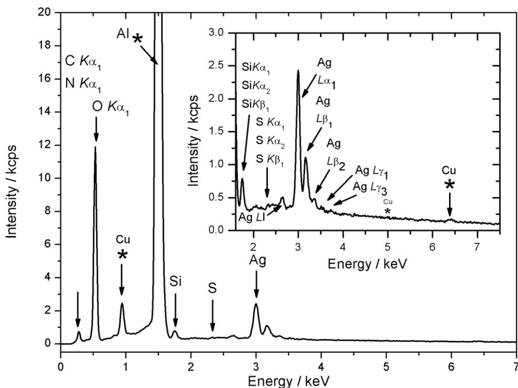
**Figure S5:** Energy-dispersive X ray spectrum from the ESPN prepared in the presence of 0.3 mol% of erbium, cast on an *aluminium* sample holder (the copper contamination arises from the sample holder) and the respective energy signal assignment.<sup>6</sup> The oxygen signal is over-estimated, as a part arises from the sample holder. The signal at around 6.4 keV in the inset should not be confused with an erbium signal. Asterisks denote the parasitic signals from copper and aluminium
