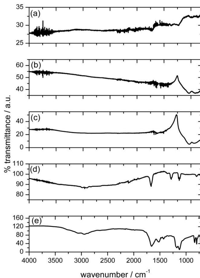
**Figure S11:** IR spectra of the ESPN: (a) prepared with 0.3 mol% Er, (b) 3 mol% Er, (c) 0 mol% Er, (d) pure peptide-coated silver nanoparticle<sup>1</sup> and (e) the peptide alone.<sup>2</sup>
