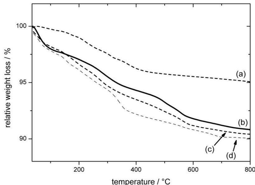
**Figure S12:** TGA curves of the (a) peptide-coated nanoparticle<sup>1</sup>, (b) Ag/peptide@SiO<sub>2</sub> nanoparticles<sup>2</sup>, (c) ESPN prepared in the presence of 3 mol% Er and (d) in the presence of 0.3 mol% Er.
