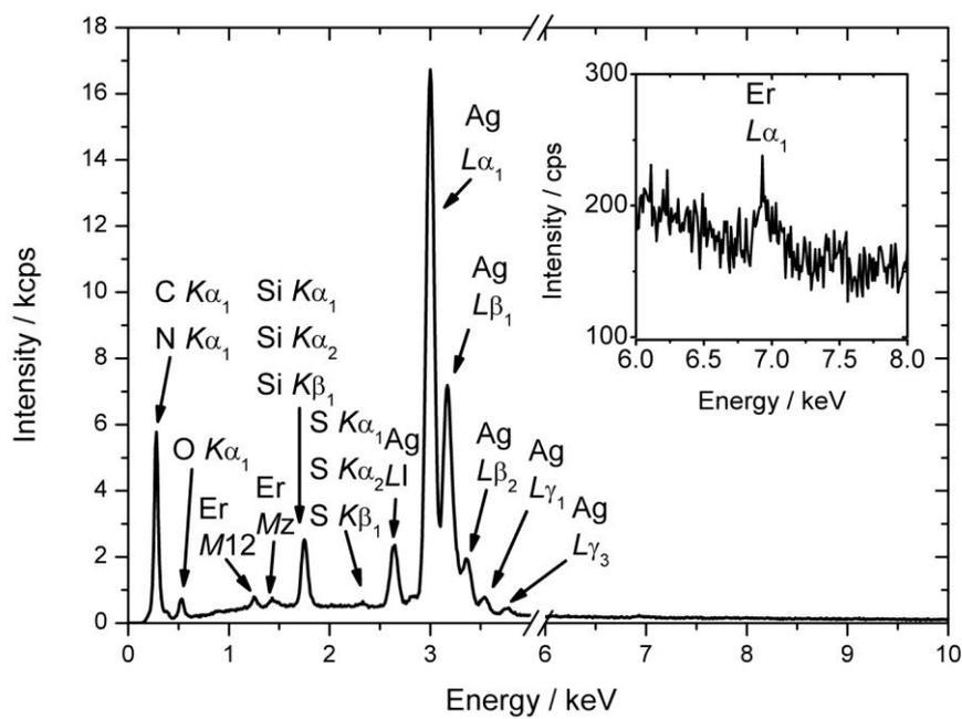
**Figure S4:** Energy-dispersive X ray spectrum from the ESPN prepared in the presence of 3 mol% of erbium, cast on a *carbon* sample holder and the respective energy signal assignment.<sup>6</sup> The carbon signal is over-estimated, as a part arises from the sample holder.
