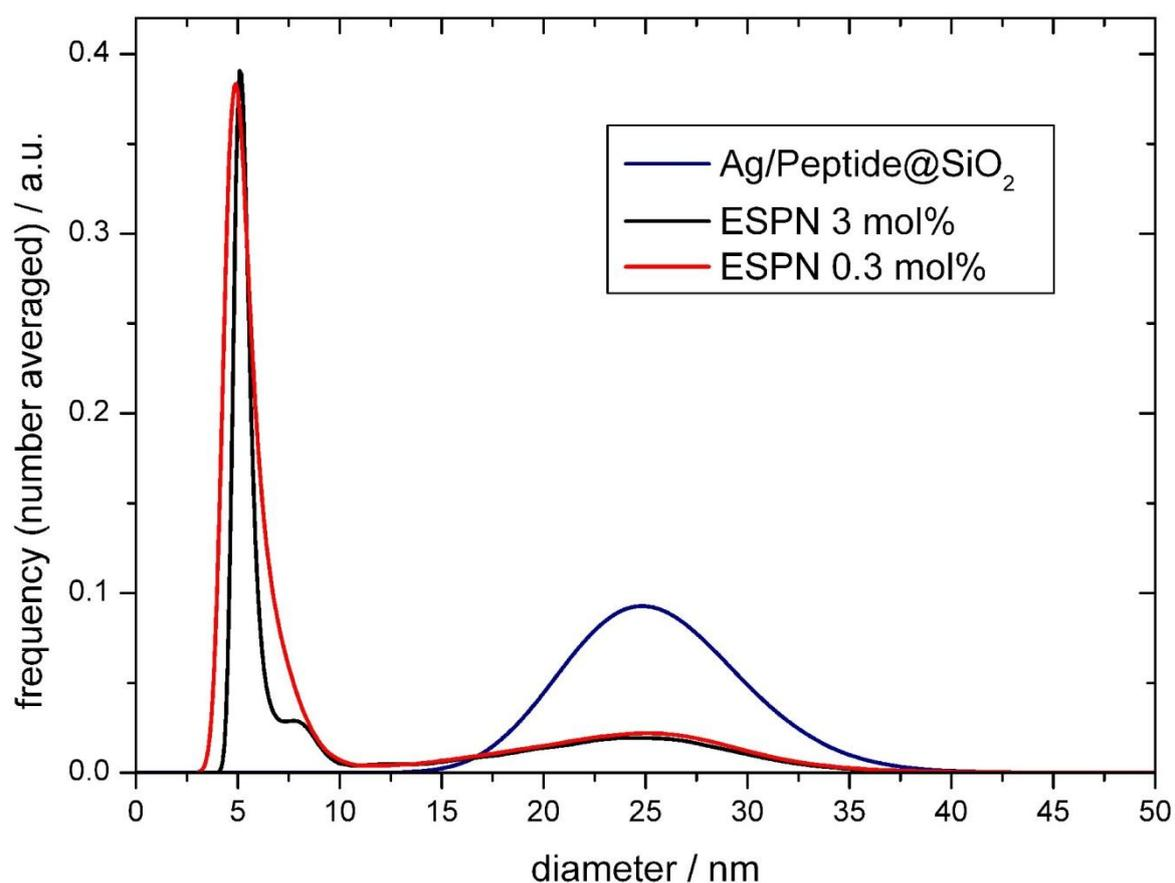
**Figure S8** Comparison of the size distribution from Ag/peptide@SiO<sub>2</sub> (blue)<sup>2</sup> and ESPN synthesized in the presence of 0.3 mol% Er (red, from TNNLS analysis) and 3 mol% Er (black, from TNNLS analysis). Note that the data are number averaged.
