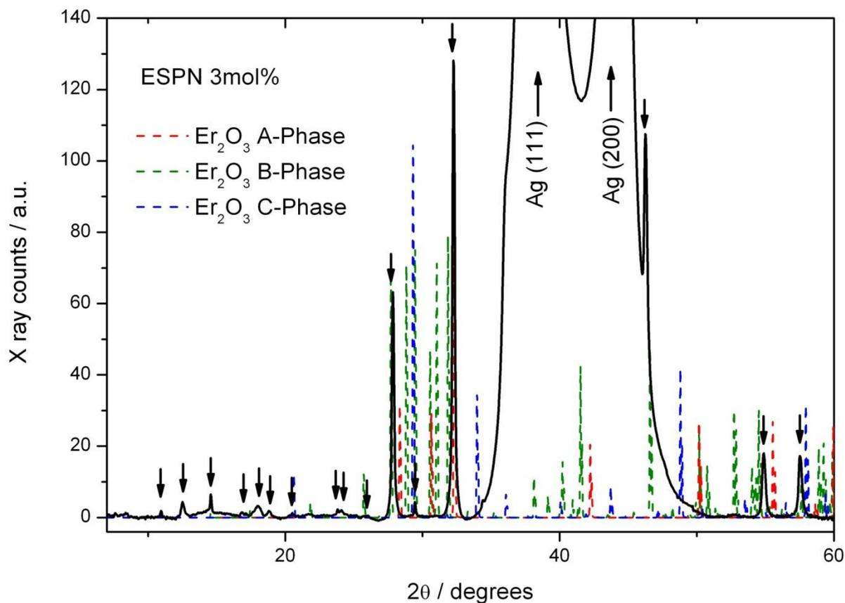
**Figure S3:** sXRD pattern of ESPN prepared with 3 mol% Er and overlay with calculated powder pattern using Fullprof<sup>3</sup> and literature data<sup>4, 5</sup>. Arrows point to the reflections arising from the erbium specie(s). Dashed lines refer to diffractogram calculated from literature data. **Table S1** lists the peak positions and the corresponding d spacings. Wavelength was 1.5456 Å
