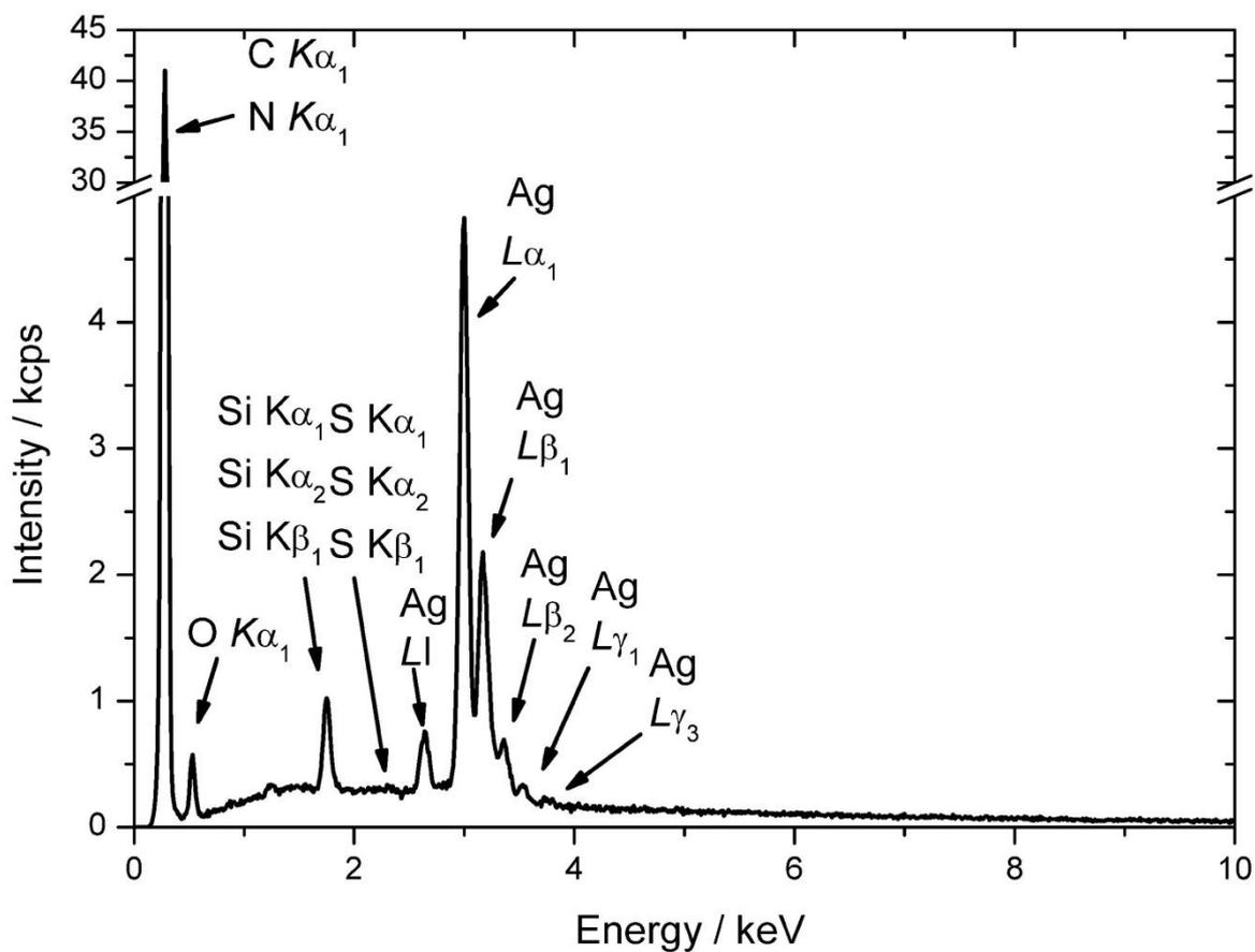
**Figure S6:** Energy-dispersive X-ray spectrum from the ESPN prepared in the absence of erbium, cast on a *carbon* sample holder and the respective energy signal assignment.<sup>6</sup> The carbon signal is over-estimated, as a part arises from the sample holder.
