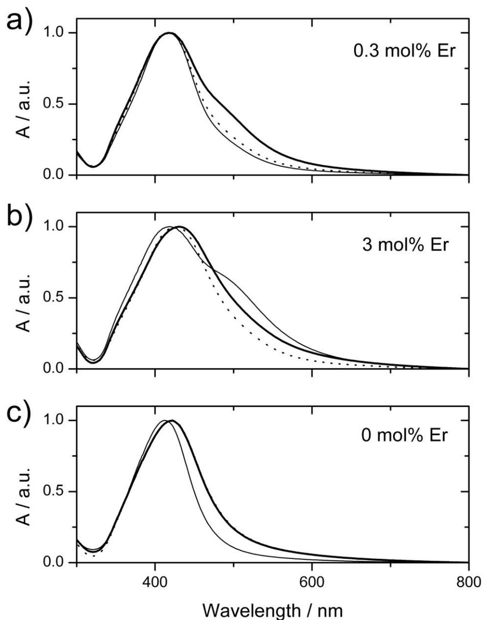
**Figure S9:** UV-Visible spectra of the ESPN grown in the presence of (a) 0.3 mol% of Er, (b) 3 mol% Er and (c) only TEOS. Thin line: after 24 hours, thick line: after 48 hours, and dotted line: after 72 hours and APTES coating. In panel (c), curves after 48 and 72 hours virtually superimpose. Data were normalized to 1 at wavelength maximum to simplify comparison.
