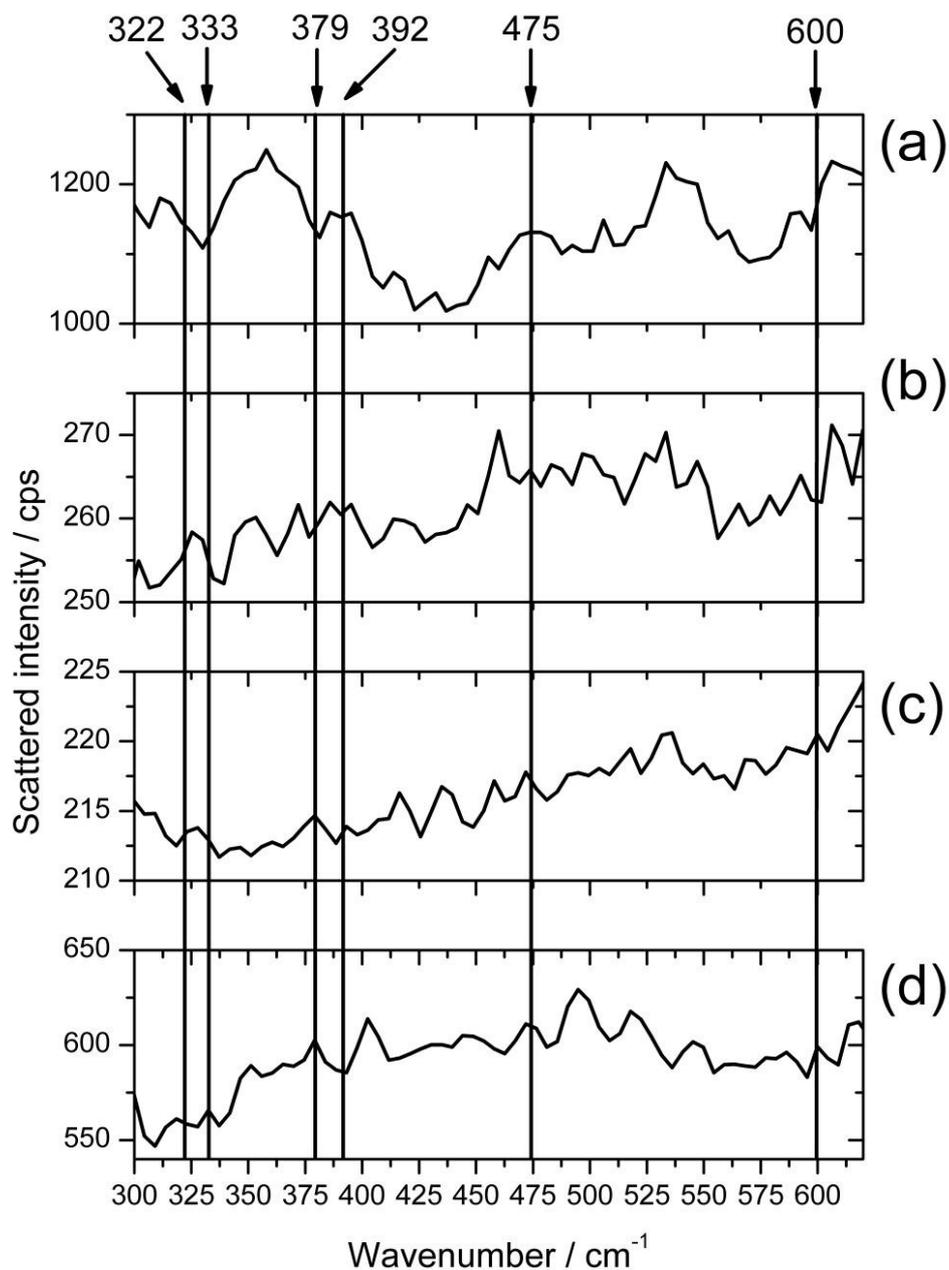
**Figure S10:** Raman spectra of (a) the pure nanoparticles, (b) ESPN prepared in the presence of 0 mol% Er, (c) 0.3 mol% Er and 3 mol% Er. Wavenumbers indicate the experimental values, compare with the published values<sup>8</sup> of 332, 338, 381, 390, 480 and 598  $\text{cm}^{-1}$  for  $\text{Er}_2\text{O}_3$ . Note the spectral similarities between all the compounds. Resolution of the CCD camera is 4  $\text{cm}^{-1}$ .
