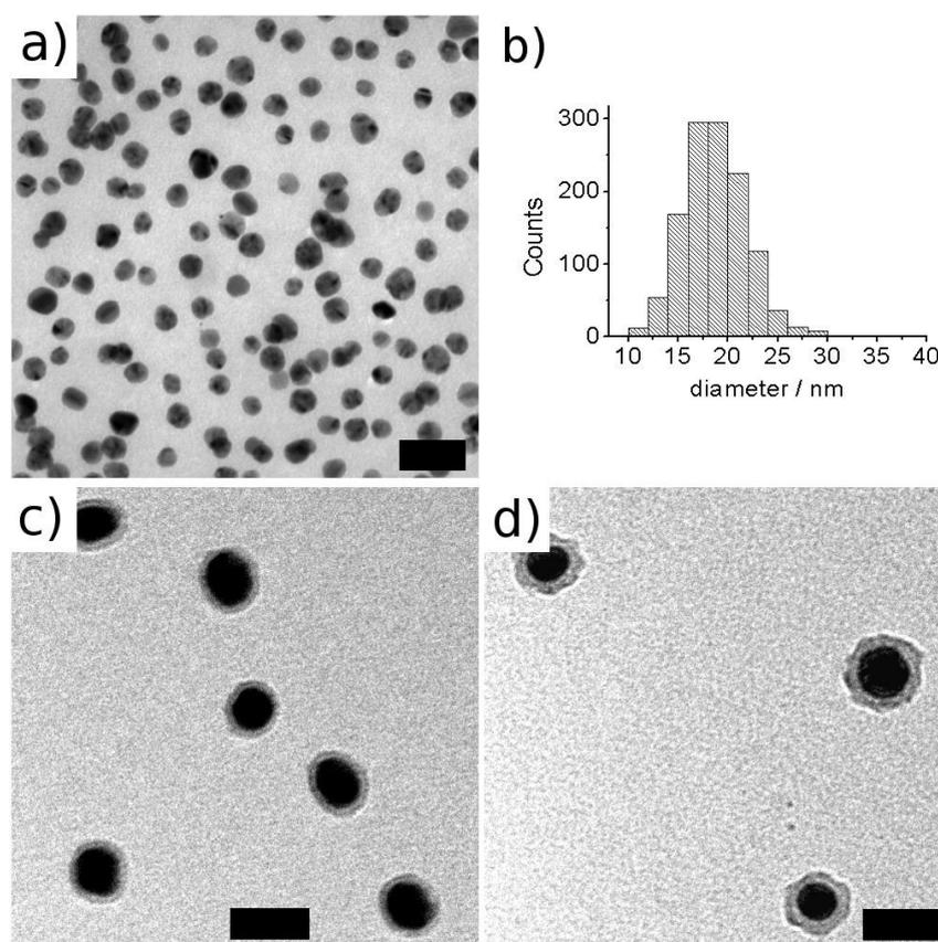
**Figure S1:** TEM of the different nanoparticles: (a) neat nanoparticles, that is, before any coating, (b) size distribution as determined from counting statistics ( $N = 1226$ , average = 18.7 nm diameter,  $\sigma = 3.2$  nm), neat nanoparticles treated with TEOS for (c) 24 hours and (d) 48 hours. Scale bar is 50 nm.
