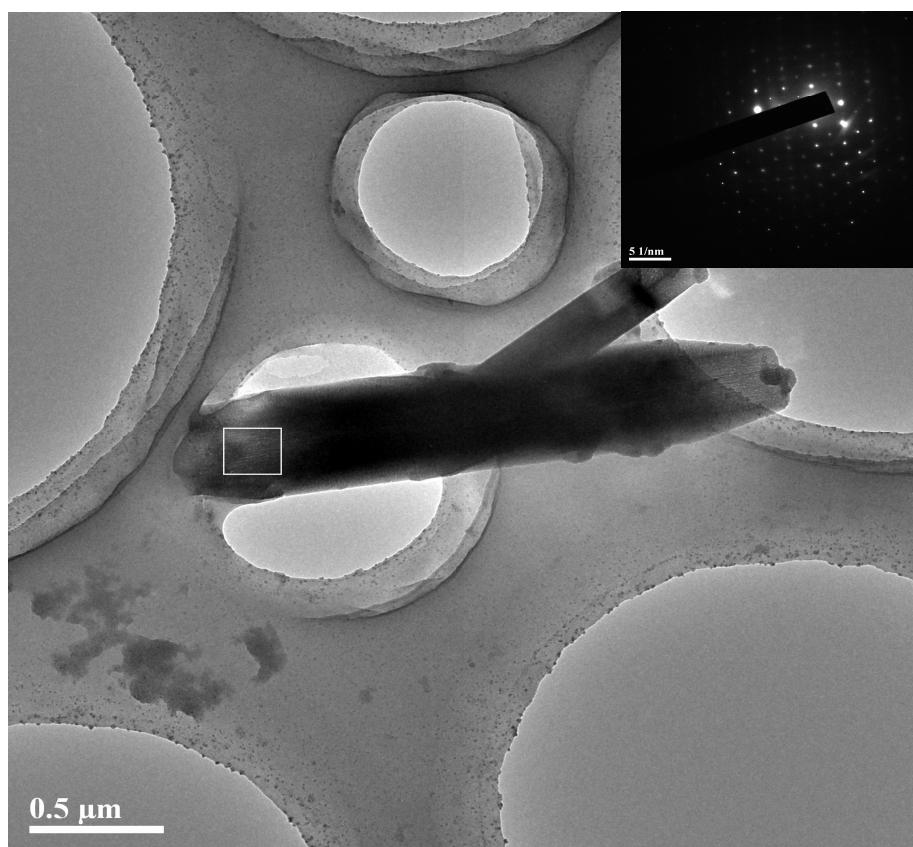
**Figure S6.** TEM image of the hexahedral rod with perfect crystal facets and the corresponding SAED pattern (inset). The highly-aligned nanotubes can be discerned at the end of the rod. The SAED pattern indicates the formation of perfect crystals with hexagonal unit cells along the crystal facet.
