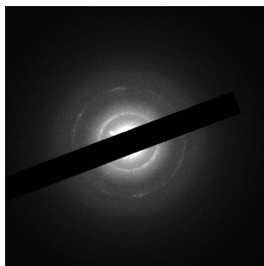
**Figure S4.** SAED pattern of pristine TNTs. The selected area is about 1  $\mu\text{m}$  in diameter and contains many nanotubes. Only diffraction rings are observed, which indicates the pristine TNTs are polycrystalline.
