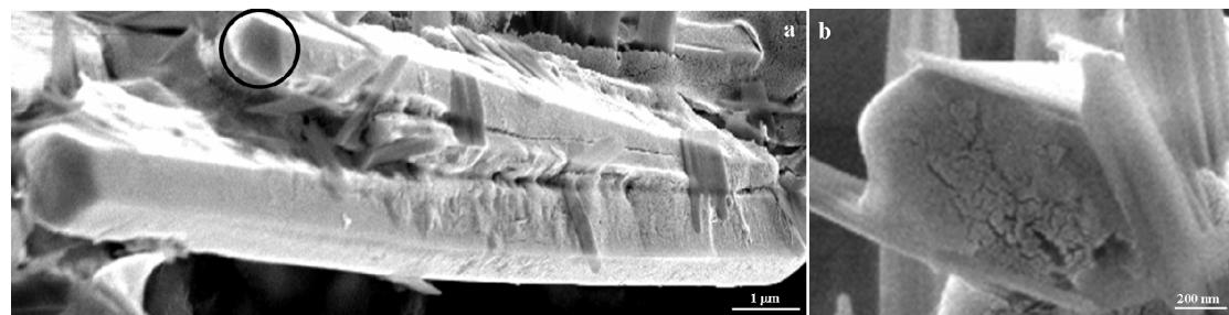
**Figure S5.** Hr-SEM image of the 3D nanotube crystals. (a) Hexahedron crystal. (b) The magnified end of the hexahedron crystal as indicated by the black circle in image a.
