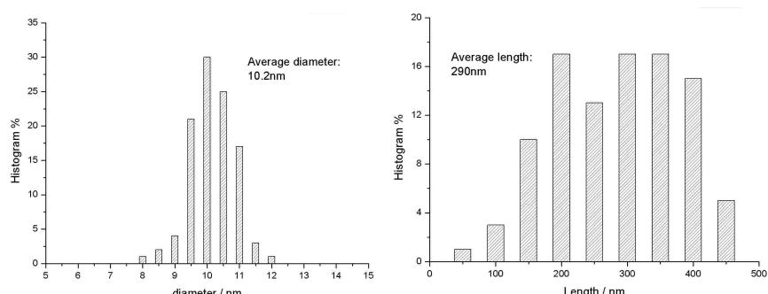
**Figure S1** Statistical diagram of size distribution of nanotube diameters and lengths.
