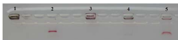
SI Fig.5 color reaction of DNA-graphene with H_2O_2 (a), H_2O_2 with TMB (b), DNA-graphene with TMB (c) and DNA-graphene in the presence of TMB and H_2O_2 (d)
