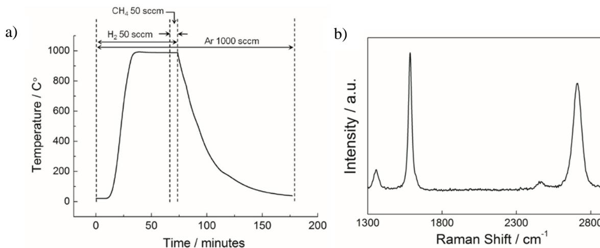
**Figure S1.** a) Temperature vs. time plot of multilayer graphene growth condition. Pressure is maintained to atmospheric pressure at all time except the initial purge stage. b) Raman spectroscopy result showing typical multilayer signal.
