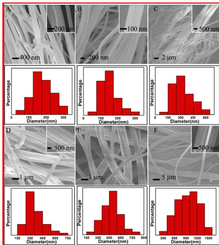
**SFigure 1.** Scanning electron microscopy and diameter distribution of the droplet elongating spun fibers under the fix temperature field (60 °C), pressures (seven times normal atmosphere) and grids (a 200 mesh filter) for samples collected at locations 180 cm away from the spray nozzle under different of the concentration of the solution:4, 7.5, 10, 12.5, 15 and 20 wt% , respectively.
