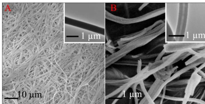
**SFigure3.** Scanning electron microscopy showing spun CuO and SiO<sub>2</sub> nanofibers without calcinations. A) CuO nanofibers. B) SiO<sub>2</sub> nanotubes. The insets are transmission electron micrograph of the nanofibers and nanotubes.
