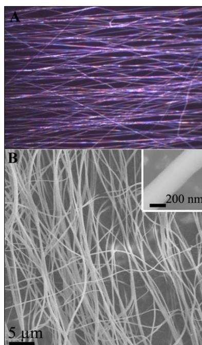
**SFigure 4** A) Optical micrographs of the aligned nanofibers suspended over the U-shaped frame, B) Scanning electron microscopy images of aligned PVP nanofibers. In order to get aligned nanofibers, the nanofibers were stretched across the gap to form a parallel array. A stainless steel U-shaped frame with a distance of 4 mm between two branches was used to transfer the aligned nanofibers by vertically moving through the gap.
