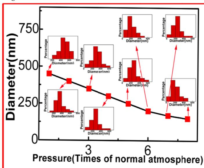
**SFigure 2.** Diameter of PVP nanofibers under a fixed square grids (a 100 mesh filter), polymer concentration (5 wt%), temperature (60 °C), for samples collected at locations 180 cm away from the spray nozzle under different pressures.
