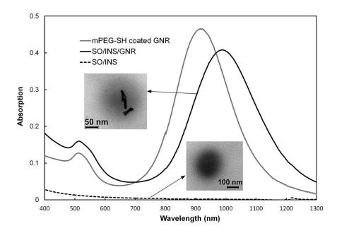
**Figure S1.** Absorption spectra and TEM images after application of the SO/INS and SO/INS/GNR formulations. The insulin concentration was increased to 3.7 mg/mL.
