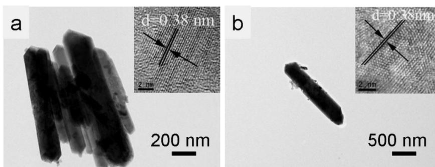
**Fig. S8.** TEM with HRTEM images of the 13-day aged nanorods prepared in (a) hexane and (b) octane, respectively.
