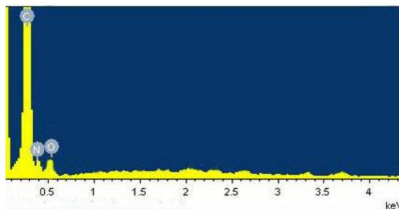
**Fig. S6.** EDS spectrum of 5-month aged layered crystals with superlattice structure in cyclohexane.
