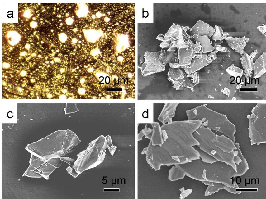
**Fig. S5.** (a,b) Microscope photograph and SEM image of 5-month aged layered crystals with superlattice structure in cyclohexane. (c,d) SEM images of 5-month aged layered crystals with superlattice structure in hexane and octane.
