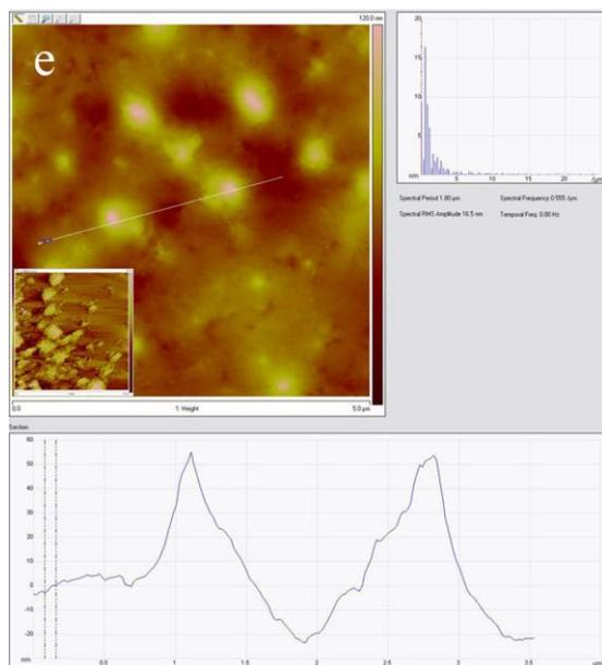
**Fig. S9.** (a-e) STM images and corresponding height profile of the 5-month aged PANI crystals with superlattice structure in (a) cyclohexane; (b) hexane; (c) octane; (d) benzene; (e) ethanol, respectively.
