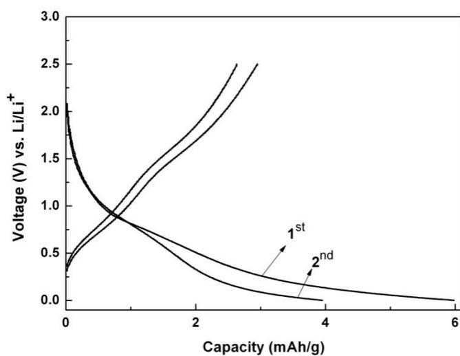
**Fig. S2** Voltage profile of pure  $\text{Ni}_3\text{Si}_2$  NR arrays grown on Ni foam for the 1<sup>st</sup>, 2<sup>nd</sup> cycle.
