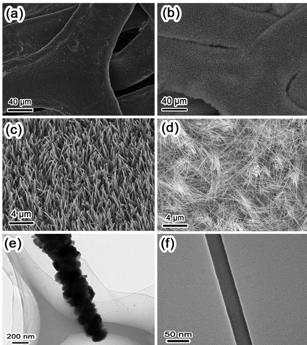
**Fig. S1** (a) SEM image of bare Ni foam. (b, c) SEM images of Ni<sub>3</sub>Si<sub>2</sub> NRs arrays grown in-situ on Ni foam with 120 sccm SiH<sub>4</sub> and 80 sccm H<sub>2</sub> at 500 °C. (d) SEM image of Ni<sub>3</sub>Si<sub>2</sub> NWs grown in-situ on Ni foam with 80 sccm SiH<sub>4</sub> and 80 sccm H<sub>2</sub> at 500 °C. (e) TEM image of Ni<sub>3</sub>Si<sub>2</sub> NR. (f) TEM image of Ni<sub>3</sub>Si<sub>2</sub> NW.
