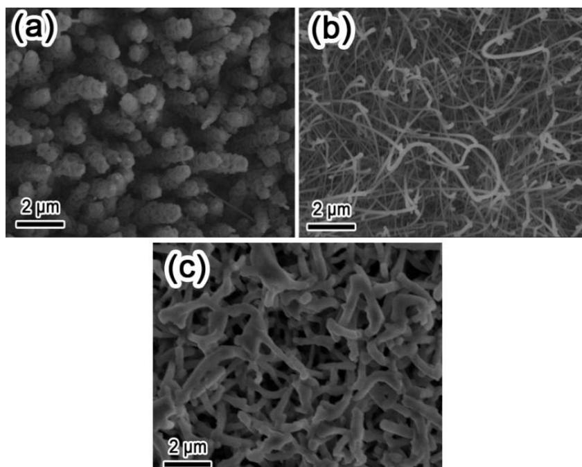
**Fig. S3** (a) SEM image of  $\text{Ni}_3\text{Si}_2/\text{Si}$  NR arrays. (b) SEM image of  $\text{Ni}_3\text{Si}_2\text{-Si}$  NWs. (c) SEM image of  $\text{Ni}_3\text{Si}_2\text{-Si}$  NWs after 100 cycles
