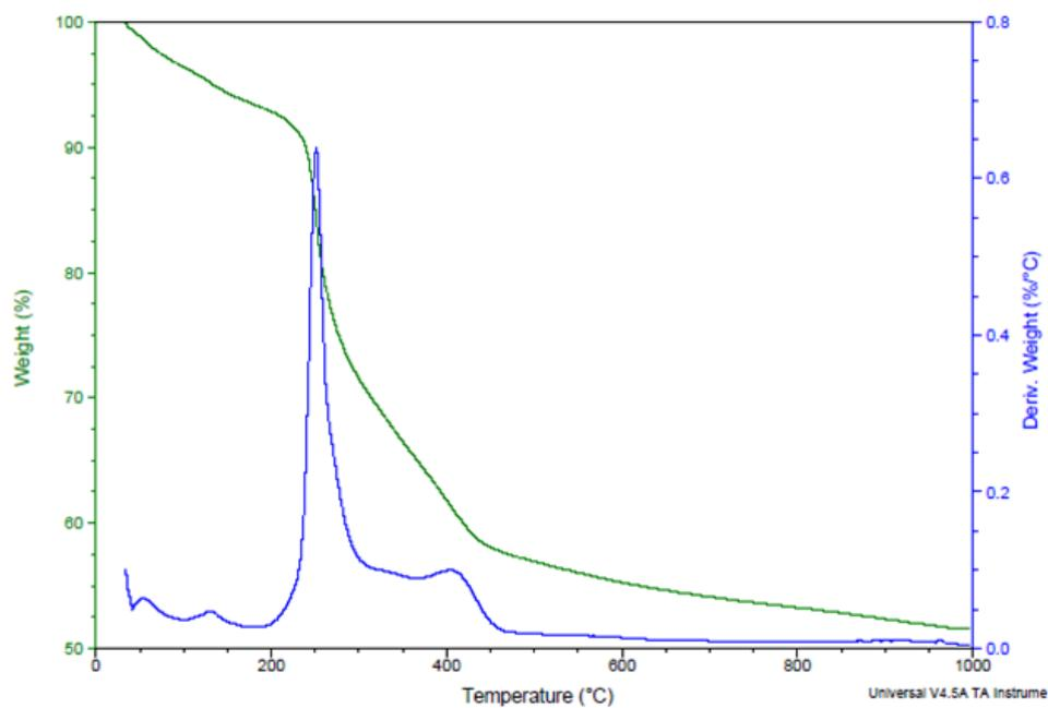
**Fig. S2.** TG/DTA analysis of L-cysteic acid terminated alumina coated silicon wafer.
