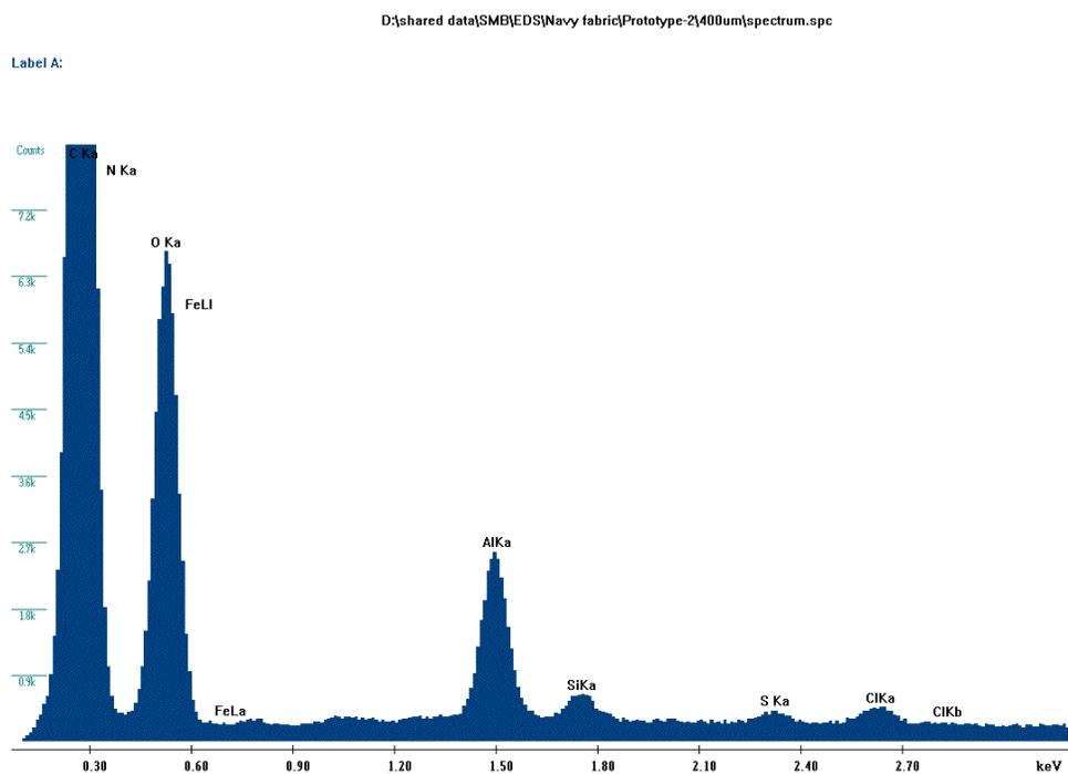
**Fig. S8.** EDX spectrum of L-cysteic acid alumoxane/ferroxane composite membrane (NPN).
