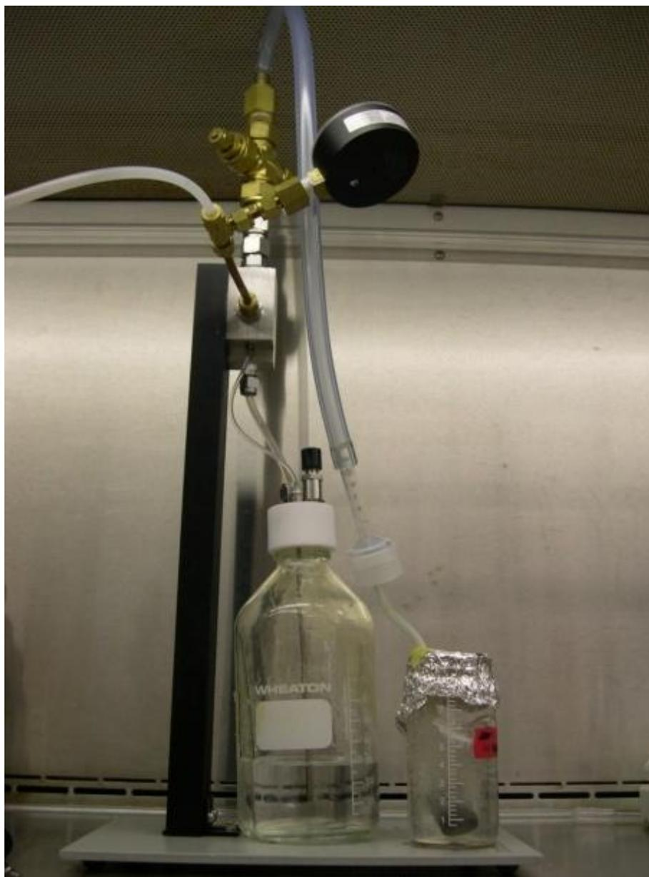
**Fig. S1.** The viral adsorption assembly.
