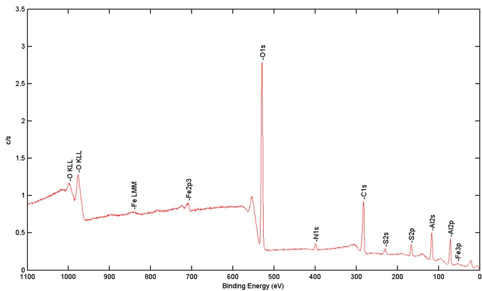
**Fig. S7.** XPS of L-cysteic acid alumoxane/ferroxane composite membrane.
