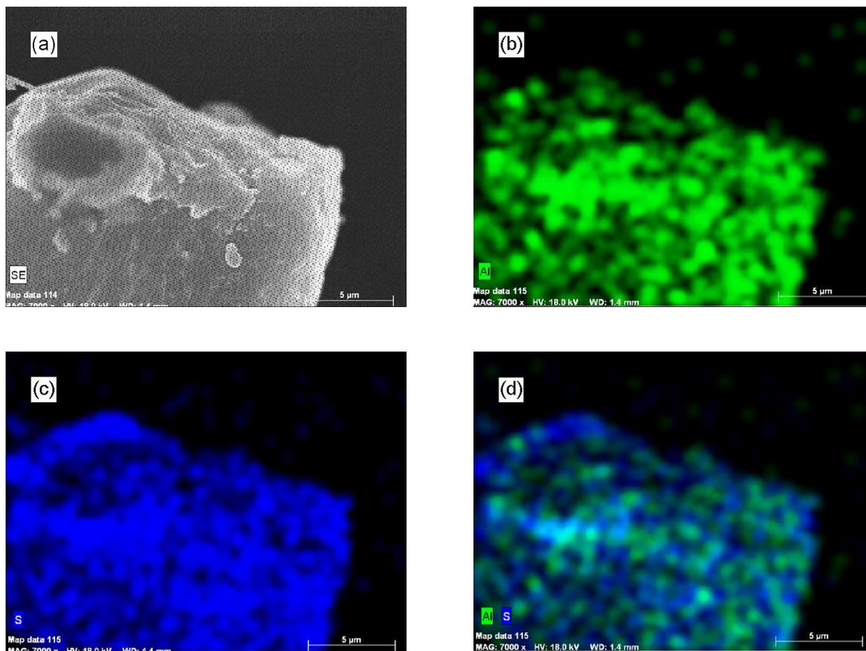
**Fig. S5.** SEM and associated EDS map of an individual alumoxane/ferroxane nanoparticle coated fiber (NPN-2x): (a) SEM image, (b) sulfur, (c) aluminum, and (d) composite of aluminum and sulfur.
