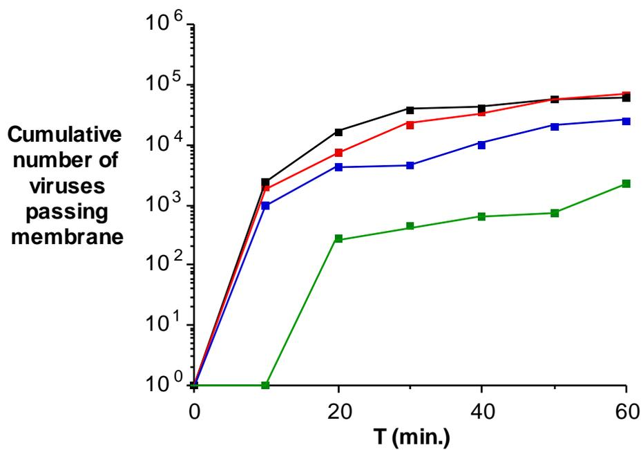
**Fig. S9.** Log plot of cumulative number of viruses passing through the Nomex<sup>®</sup>-derived filters as a function of exposure time for MS2 bacterage adsorption studies: untreated Nomex<sup>®</sup> (■), alumoxane-ferroxane (■), alumoxane-ferroxane XXX (■), and alumoxane-ferroxane XX heated to 160 °C for 2 hours (■).
