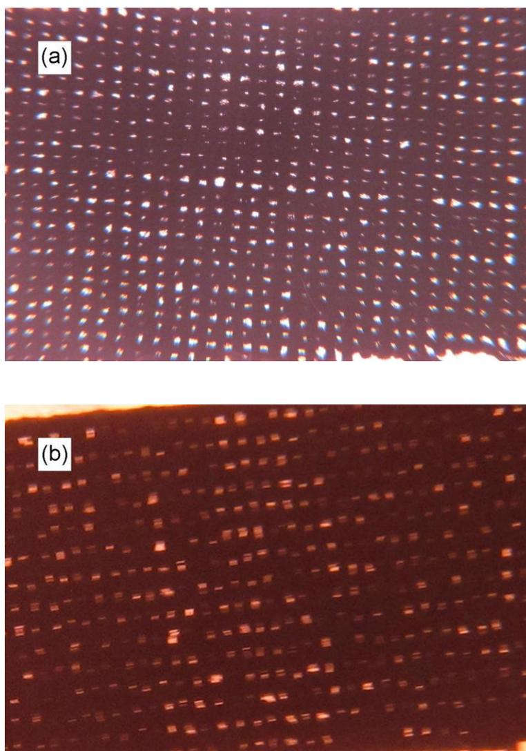
**Fig. S10.** Optical images of (a) Nomex<sup>®</sup> fabric and (b) L-cysteic acid alumoxane functionalized Nomex<sup>®</sup> fabric. Adapted from S. J. Maguire-Boyle and A. R. Barron, *J. Membrane Sci.*, 2011, **382**, 107-115.
