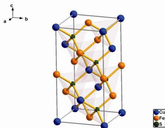
**Fig. S1** Three-dimensional illustration of unit cell for chalcopyrite  $\text{CuFeS}_2$ .
