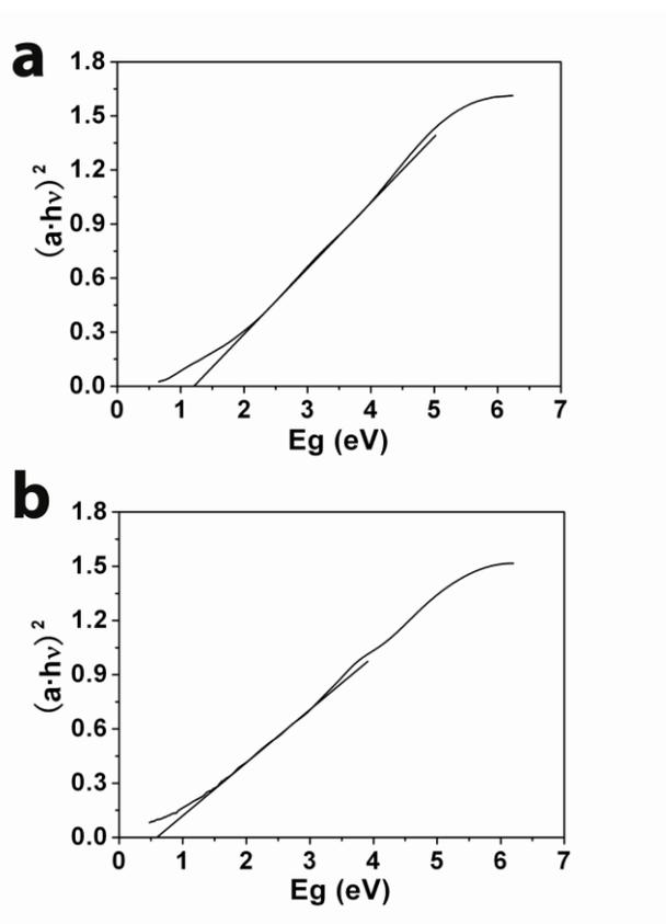
**Fig. S2** Plot of  $(a \cdot hv)^2$  versus photon energy. (a)  $(a \cdot hv)^2$ - $E_g$  spectrum of CuFeS<sub>2</sub> nanoparticles. Extrapolation of the linear region shows a band gap of 1.20 eV. (b)  $(a \cdot hv)^2$ - $E_g$  spectrum of bulk chalcopyrite powders. Extrapolation of the linear region shows a band gap of 0.59 eV.
