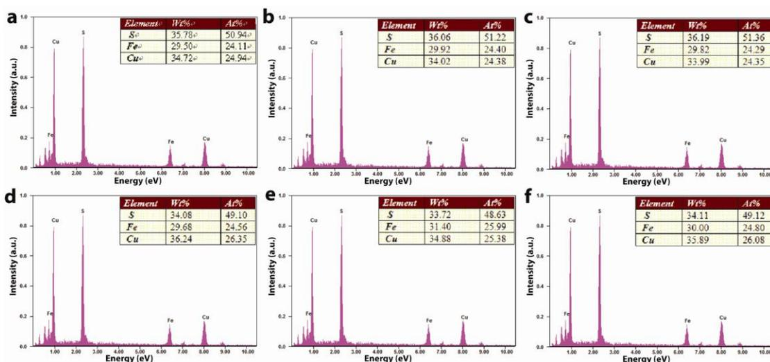
**Fig. S4** EDX spectra of CuFeS<sub>2</sub> nanoparticles. (a-c) EDX spectra of the as-synthesized CuFeS<sub>2</sub> nanoparticles. (d-f) EDX spectra of CuFeS<sub>2</sub> nanoparticles after thermoelectric measurements.
