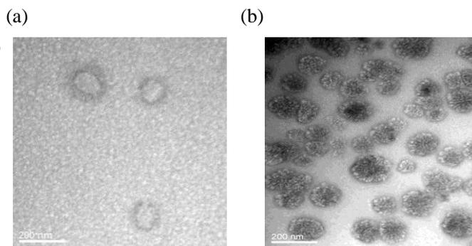
Figure S4. TEM image of (a) pure liposomes and (b) TSMLs at 42 °C.
