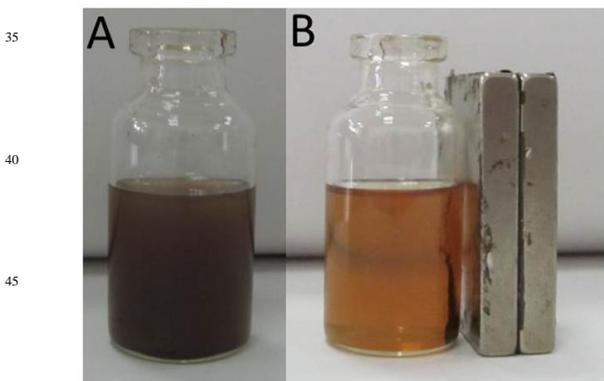
Figure S2. Optical photos of TSMLs respond to a magnetic field: A. TSMLs are black without a magnetic field; B. TSMLs are separated in a magnetic field.
