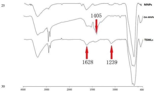
Figure S1. FTIR spectra of MNPs, OA-MNPs and TSMLs.
