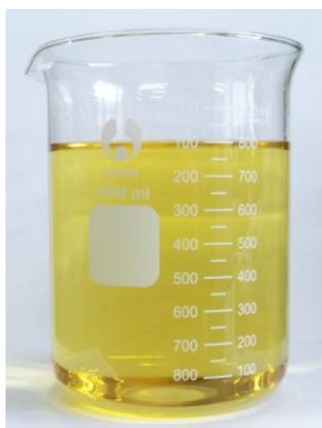
Fig. S1 The digital photograph of CDs solution (one-pot synthesis) after centrifugation at 8000 rpm. The upper volume of the beaker is 1000 mL. For large-scale preparation of CDs in one pot, 7.0448 g ascorbic acid was dissolved in water (760 mL) to form a clear solution, followed by adding a Cu(Ac) 2 solution (40 mL, 0.1 M). After centrifugation at 8000 rpm, the solvent of suspension was removed with the aid of a rotary evaporator. Then the final sample was obtained by vacuum drying at 60 °C. The CDs with measured weight up to 6.2 g was obtained in one pot.
