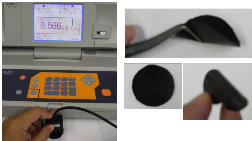
Figure S1. Conductivity test of SEBS/SWCNTs film; it can be bended or folded.
