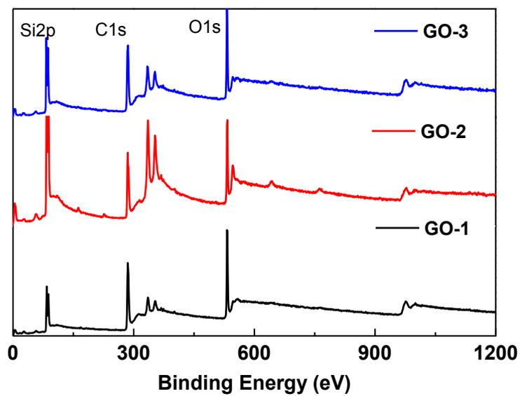
**Figure S2.** Wide-scan XPS spectra of graphene oxide samples (GO-1, GO-2 and GO-3).
