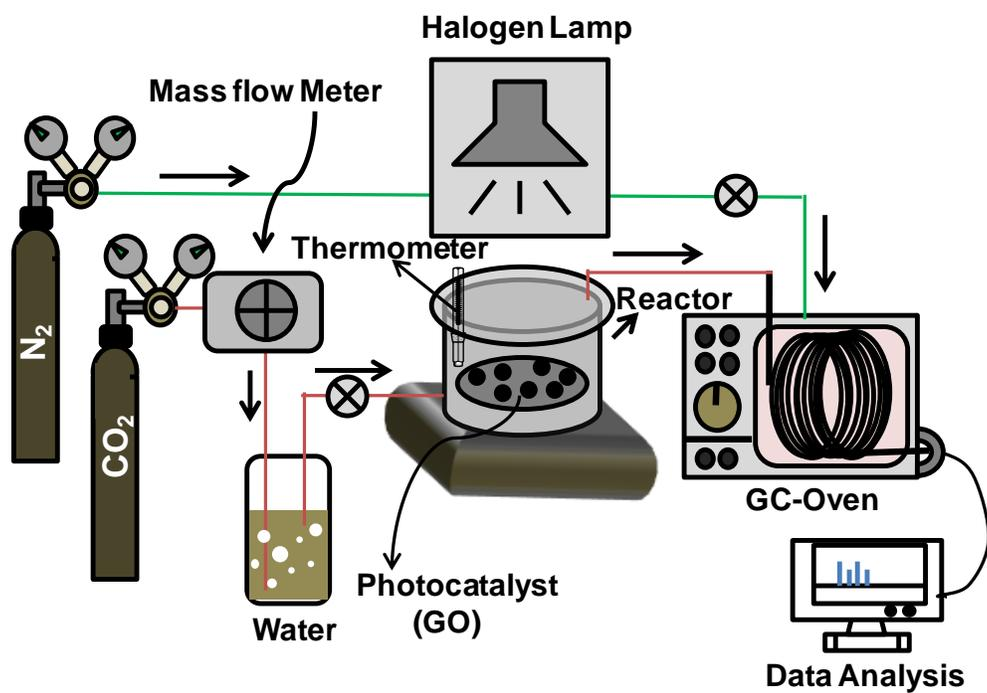
**Figure S1.** Schematic diagram of the photocatalytic reduction of CO<sub>2</sub> with graphene oxide.
