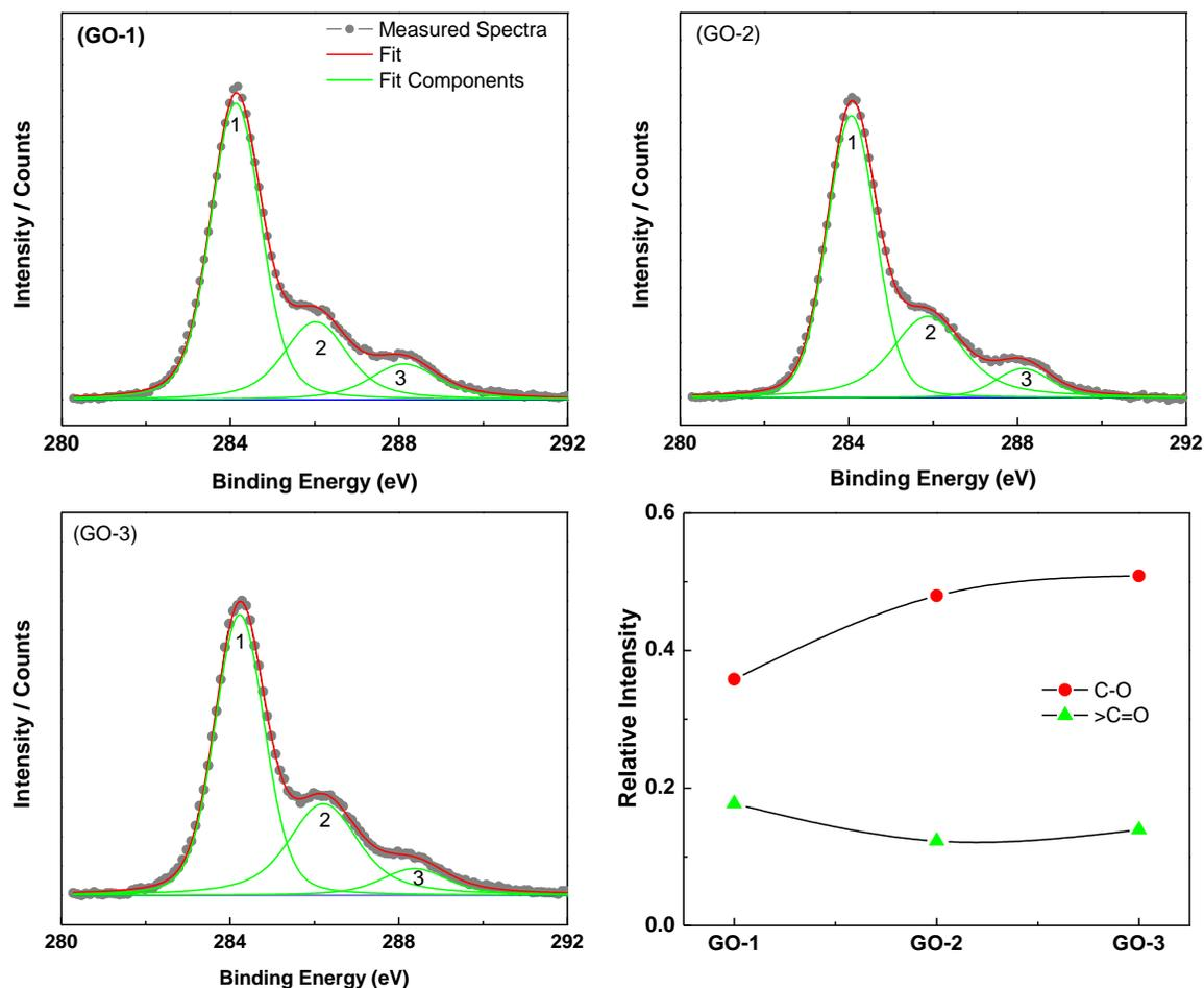
**Figure S4.** XPS spectra (C1s) with deconvoluted peaks of graphene oxide samples (GO-1, GO-2 and GO-3) after photocatalytic reaction. Peaks 1 to 3 represents C=C (or sp<sup>2</sup>), C-O and >C=O components, respectively. Relative areal intensity of -C-O and >C=O normalized with sp<sup>2</sup> components.
