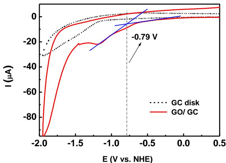
**Figure S3.** Cyclic voltammograms of glassy carbon and reduction onset potential of GO film casted onto a GC electrode in acetonitrile containing 0.1 M TBAP (tetrabutylammonium tetrafluoroborate). Scan rate = 100 mV/s. (Counter electrode: Pt )
