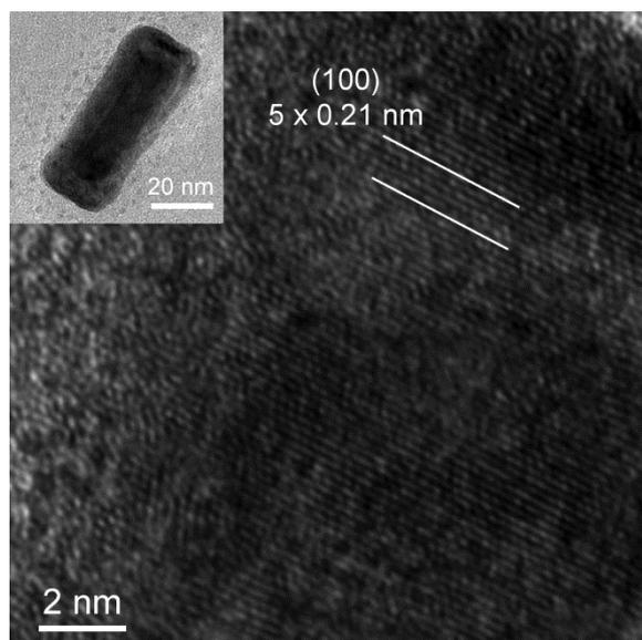
**Fig. S2** HRTEM image of a Au–Pd bimetallic nanostructure from the sample grown with the SC Au NRs as the seeds. The inset is the nanostructure on which the HRTEM image was acquired. The sample was grown with 0.18 mL of  $\text{H}_2\text{PdCl}_4$  (0.01 M).
