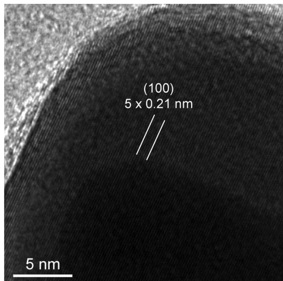
**Fig. S1** HRTEM image of a Au–Ag bimetallic nanostructure from the sample grown with the SC Au NRs as the seeds. The sample was grown with 0.48 mL of  $\text{AgNO}_3$  (0.01 M).
