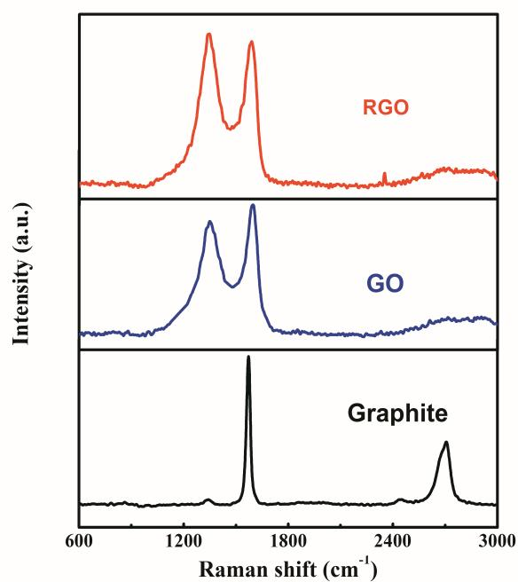
**Fig.S2** Raman spectrum of graphite, GO and RGO
