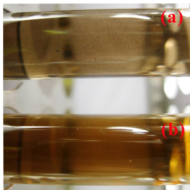
**Fig.S5** Photographs of (a) GO/DMSO dispersion (0.05 mg/mL) with solid GO dispersed by direct sonication; (b) GO/DMSO dispersion (0.05 mg/mL) obtained by the method of solution-exchange
