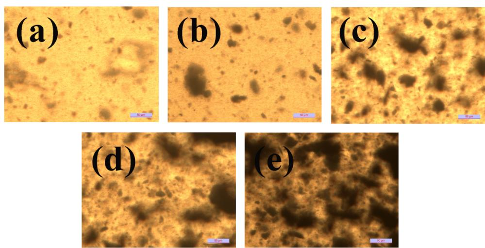
**Fig.S6** Optical microscopic images of RGO/PMMA containing 0.1 wt% (a), 0.3 wt% (b), 0.5 wt% (c), 0.7 wt% (d) and 1 wt% (f) of ANFGS
