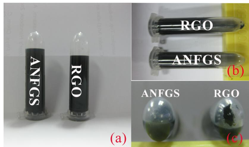
**Fig.S3** (a): The dispersions of ANFGS (0.5 mg/mL) and RGO (0.5 mg/mL) with sonication of 2 h, (b) and (c): The dispersion state of ANFGS and RGO in NMP solution after centrifuging for 10 min at 3000 rpm
