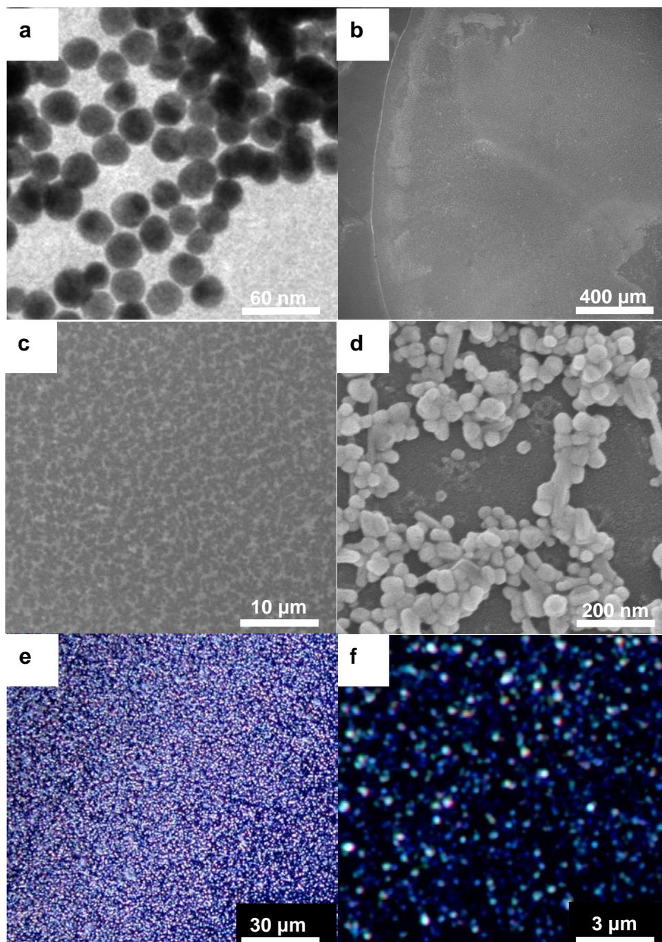
**Fig. S1** (a) TEM image of the prepared Ag nanoparticles. (b), (c), (d) SEM images of the prepared Ag nanoparticles film by dropping casting. The large area of Ag nanoparticle film contains a dense collection of Ag aggregates consisting of many Ag-NPs. (e), (f) Dark-field photographs of the prepared Ag nanoparticles on a glass slide obtained under optical microscopy. Each bright spot represents the Ag aggregate.
