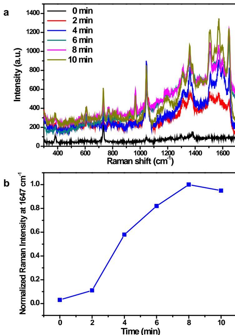
**Fig. S2** (a) Time-dependent SERS measurement of the Hantzsch reaction of formaldehyde, taken every 2 min at 457 nm. (b) Temporal evolution of SERS intensity at 1647 cm<sup>-1</sup> of DDL. The mixture was refluxed at 60 °C in water bath. All of the concentration is 1 nM. The Raman intensity increased during the first few minutes and reached its maximum at about 8 min. Accordingly, to obtain the maximum SERS efficiency, all of the formaldehyde aqueous solutions in this work
