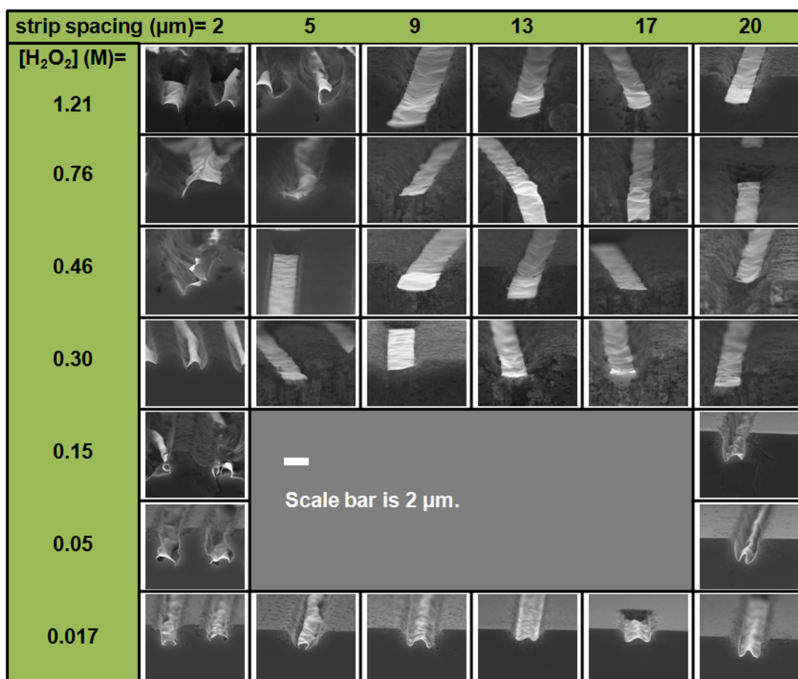
Fig. S3. Cross-sectional SEM images of the etched samples used to construct the stability diagram in Fig. 11 in the main text. [\text{HF}] was fixed at 1.73 M.
