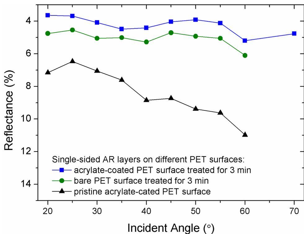
**Fig. S4** Effects of the angle of incidence at a wavelength of 600 nm on the AR characteristics of PET substrates overcoated with 90 nm-thick silica nanoparticle AR layers. The AR layers were coated on three different PET surfaces: (i) an acrylate-coated PET surface that was plasma-treated for 3 min, (ii) a bare PET surface that was plasma-treated for 3 min, and (iii) a pristine acrylate-coated PET surface without any plasma pretreatment.
