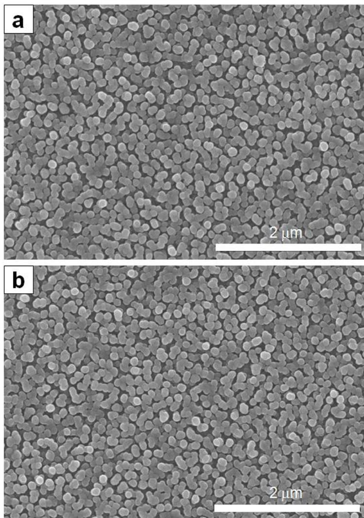
**Fig. S5** FE-SEM images of a 90 nm-thick silica nanoparticle AR layer coated on an acrylate-coated PET surface that was plasma-treated for 3 min (a) before and (b) after exposing the AR layer to 3000 cycles of curvature-imposed tensile strain.
