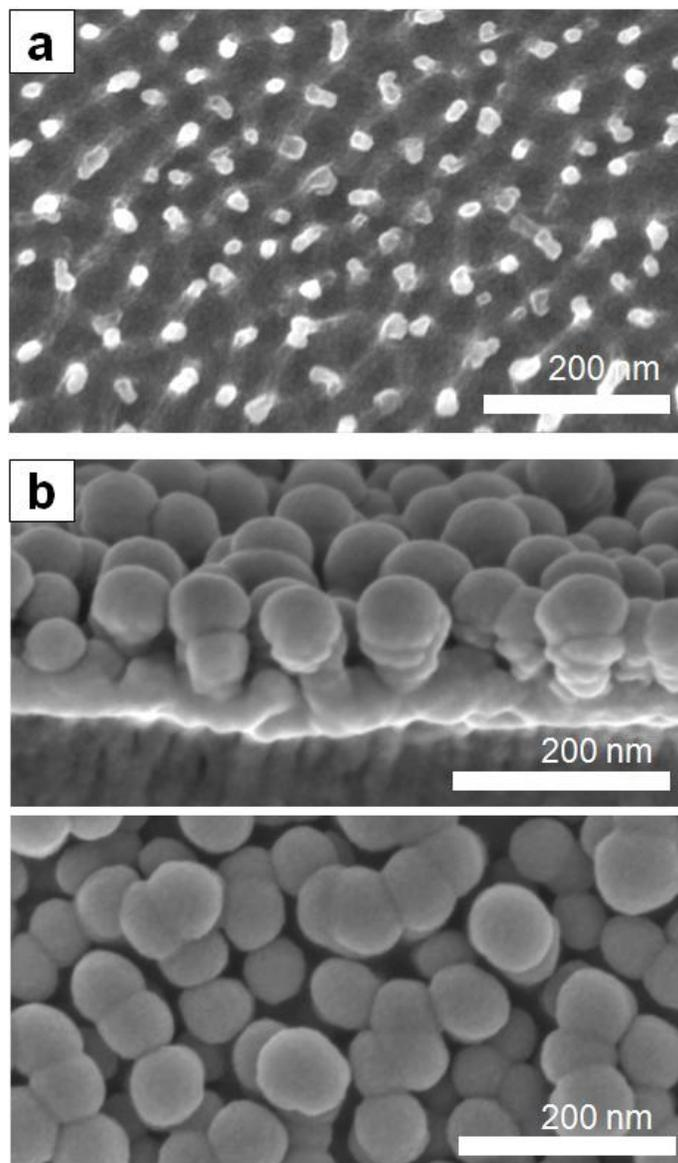
**Fig. S3** FE-SEM images of (a) polymer protrusions developed on a 3 min-treated bare PET surface and (b) 90 nm-thick silica nanoparticles coated subsequently on the bare PET surface.
