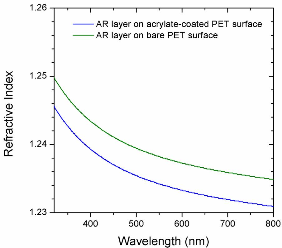
**Fig. S1** Refractive indices of 90 nm-thick silica nanoparticle AR layers coated on acrylate and bare PET surfaces pretreated for 3 min.
