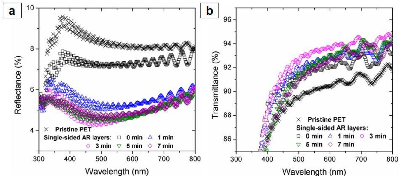
**Fig. S2** (a) Specular reflection and (b) transmission spectra of 90 nm-thick silica nanoparticle AR layers coated on bare PET surfaces pretreated for different times. The bare PET surfaces were treatment time
