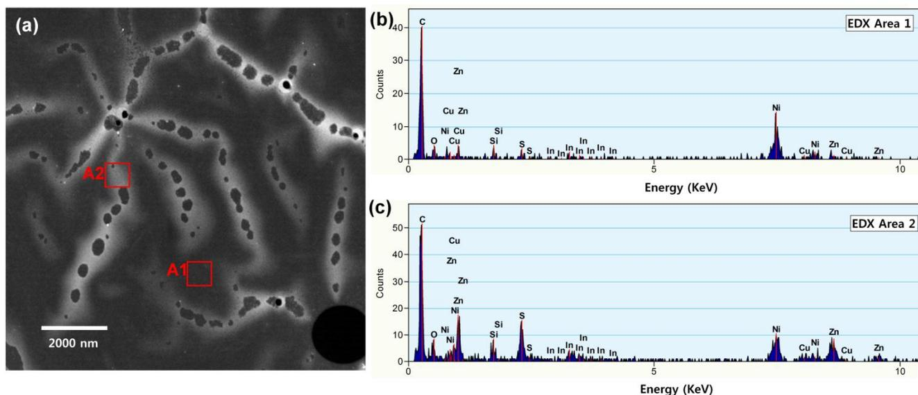
**Fig. S2** For element analysis, FEI instrument with a field emission gun was operated at 300 kV, equipped with an EDAX spectrometer with Si (Li) detector. In dark-field STEM images of QDs (a), the bright area indicates the self-assembled QDs, and dark area exhibits nickel holey carbon support grid of the sample confirmed by EDX data (b) and (c). It clearly shows that 1D like self-assembled property of as-synthesized QDs.
