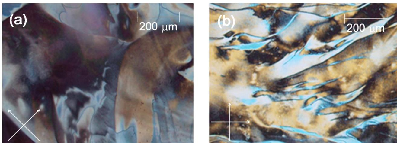
**Fig. S5** Schlieren textures were shown in both negative (a) and positive (b) dielectric anisotropic LCs on ITO surfaces without alignment layers
