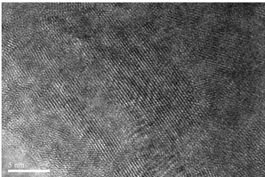
**Figure S5-3** HRTEM image of synthesized NaYF<sub>4</sub>:Yb<sup>3+</sup>/Ho<sup>3+</sup> nanocrystals: HRTEM image shows NaYF<sub>4</sub>:Yb<sup>3+</sup>/Ho<sup>3+</sup> nanocrystals have clear and continuous fringe lattice.
