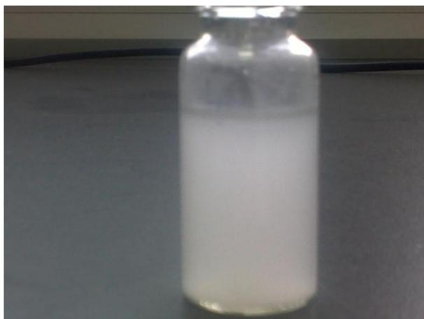
**Figure S13.** Photonic image of  $0.1 \text{ g}$   $\text{NaGdF}_4:\text{Yb}^{3+}/\text{Er}^{3+}$  nanorods dispersed in  $10 \text{ mL}$  deionized water.
