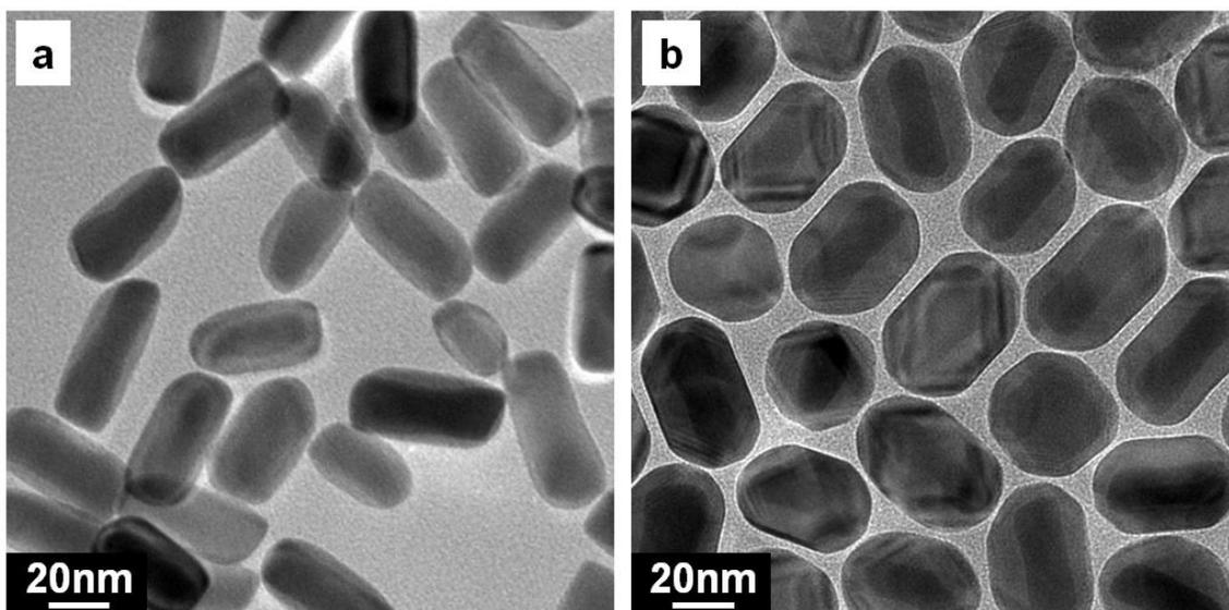
**Fig. S1** TEM images of AuNR@Ag nanoparticles with different silver shell thicknesses. The surfaces of AuNRs were coated with silver shells having thicknesses of (a) 5 nm and (b) 11 nm, obtained by adjusting the amount of AgNO<sub>3</sub> to 0.001 mmol and 0.01 mmol, respectively.
