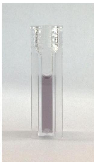
**Fig. S4** Photograph of the rattle-structured AuNR@SiO<sub>2</sub> dispersed in aqueous solution.
