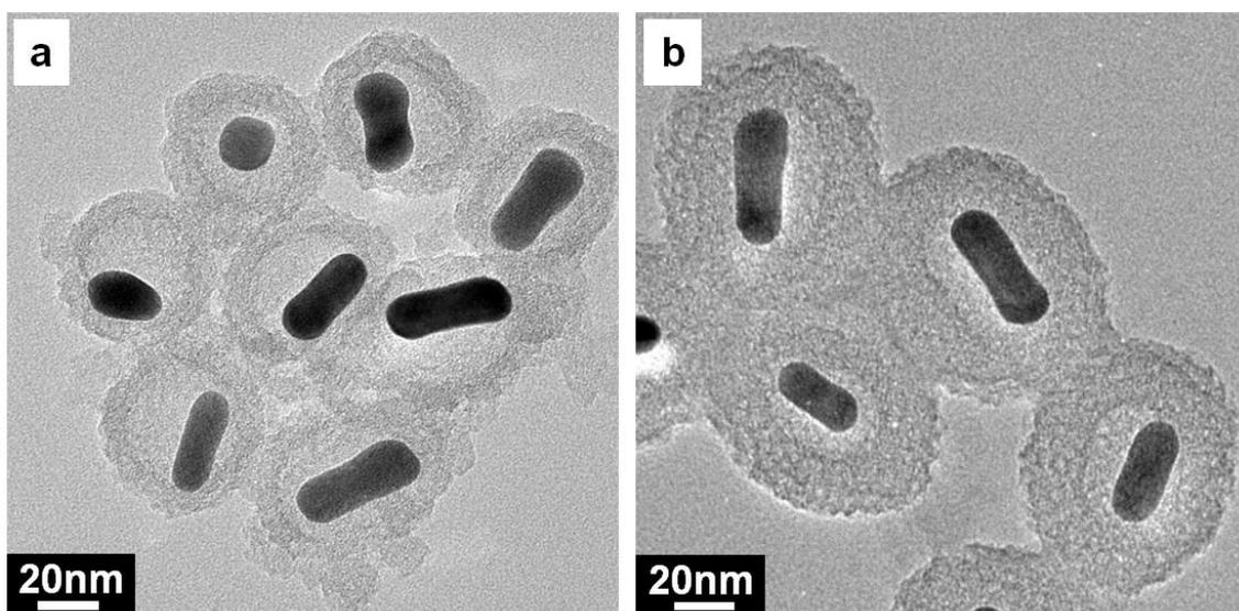
**Fig. S2** TEM images of rattle-structured AuNR@mSiO<sub>2</sub> with different SiO<sub>2</sub> thicknesses. The shell thicknesses of (a) 8 nm and (b) 21 nm were obtained at TEOS concentrations of 0.04 mmol and 0.08 mmol, respectively.
