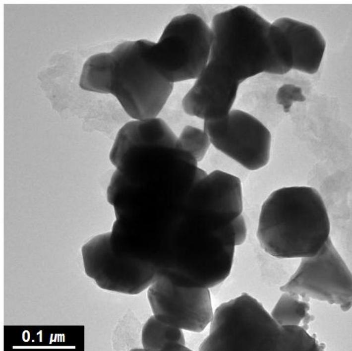
**Fig. S5** TEM image of nanoparticles regrown from AuNRs without silica nanocapsules.
