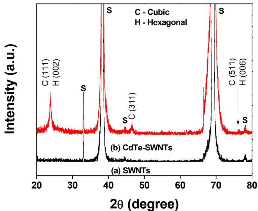
Fig. S2. XRD patterns of undeposited and CdTe-deposited SWNTs. The CdTe NPs were electrodeposited at  $-0.50$  V vs. Ag/AgCl with a charge density of  $2000$  mC/cm<sup>2</sup>. (S: SWNT/gold/Si substrate)
