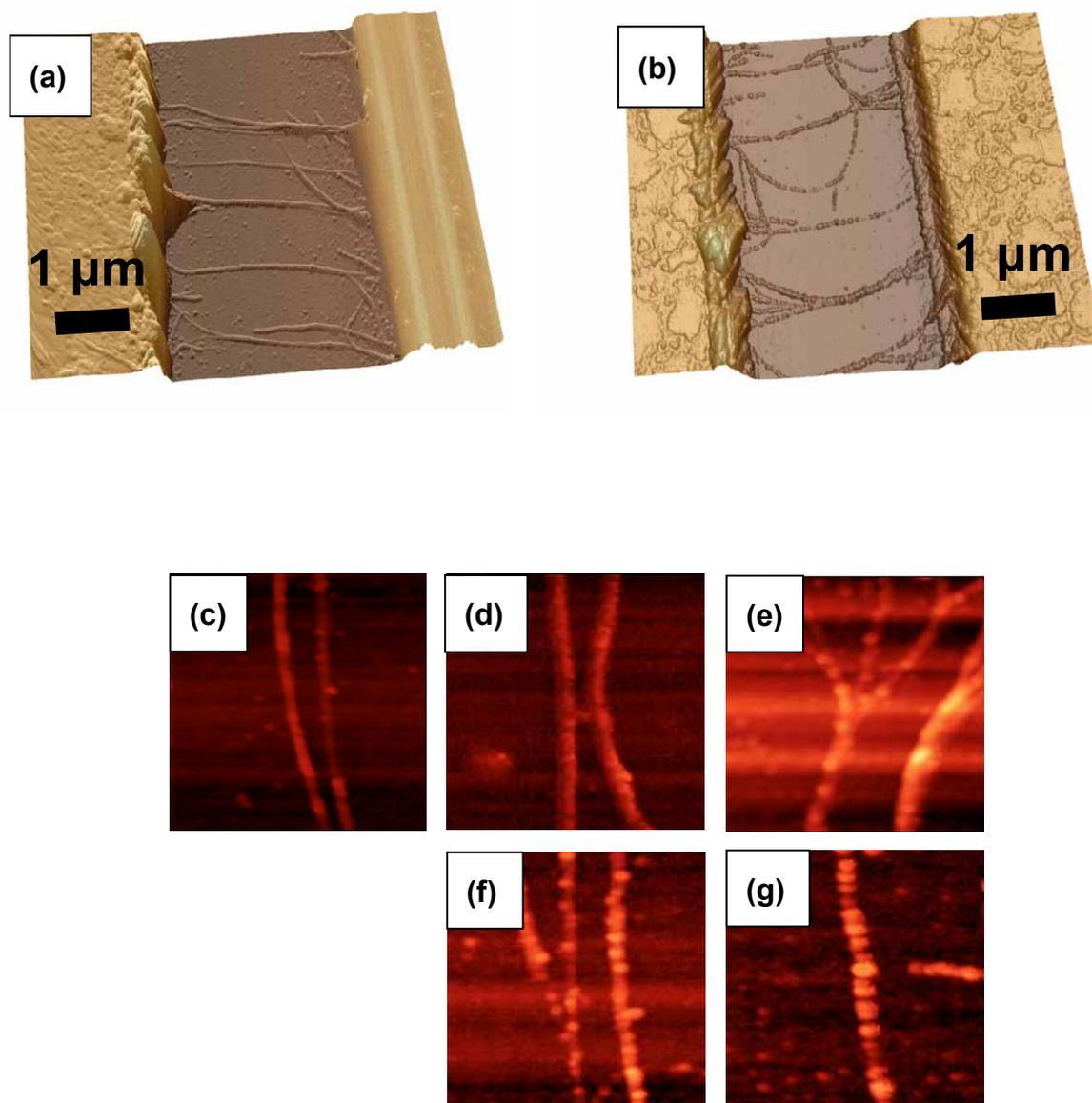
Fig. S1. AFM images of (a) undeeposited and (b) deposited SWNTs between gold electrodes with CdTe ( $30 \text{ mC/cm}^2$ ). The topography of (c) bare and (d–g) CdTe/SWNT hybrid nanostructures. The CdTe was electrodeposited at fixed  $-0.50 \text{ V}$  vs. Ag/AgCl with varying charge densities: (d) 5, (e) 10, (f) 20, and (g)  $30 \text{ mC/cm}^2$ .
