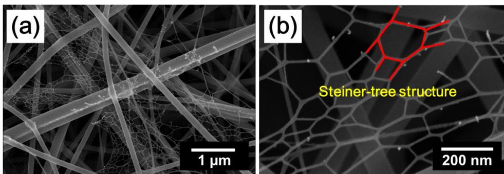
**Fig. S2** (a) Low and (b) high magnification FE-SEM images of PMIA nanofibers showing the Steiner-tree structure.
