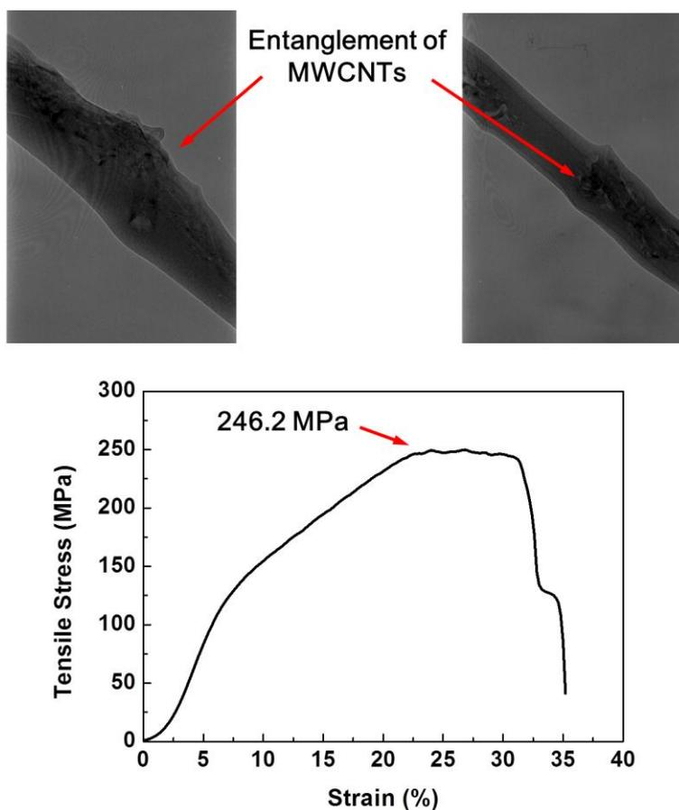
**Fig. S3** TEM images and stress-strain curve of PMIA/MWCNT nanofibers with MWCNTs contents of 2 wt%.
