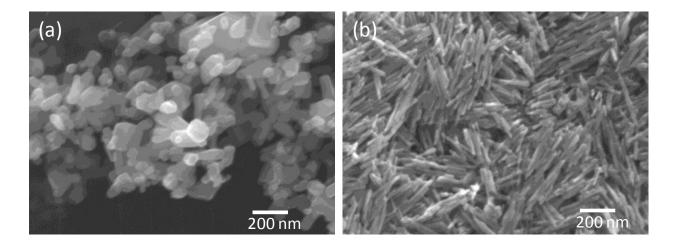
Figure S1: SEM images of commercial ZnO nanoparticles (Sigma Aldrich, product number: 544906) and synthesized ZnO nanorods.
