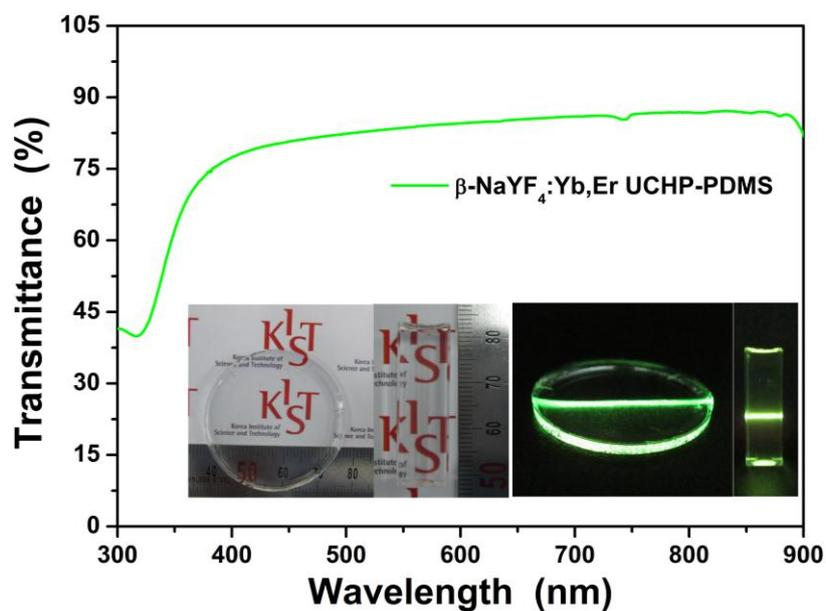
**Figure S9.** Transmittance spectrum of  $\beta$ -NaYF<sub>4</sub>:Yb,Er upconversion hexagonal prism (UCHP)-PDMS composite. Inset shows prepared UCHP-PDMS disk and bar under room light (left) and under NIR laser (right).
