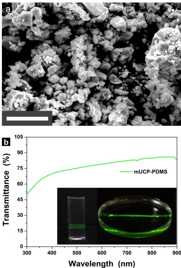
**Figure S10.** (a) Scanning electron microscopy image of micrometer-sized upconversion phosphor (mUCP) and (b) transmittance spectrum of mUCP-PDMS composite. Inset shows prepared mUCP-PDMS bar (left) and disk (right) under NIR laser. Scale bar represents 10  $\mu\text{m}$ .
