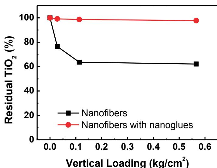
**Fig.S2** Adhesion test using peeling off TiO<sub>2</sub> films with a PDMS stamp.
