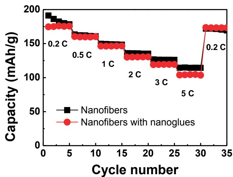
Fig.S5 Rate capability of  $\text{TiO}_2$  batteries.
