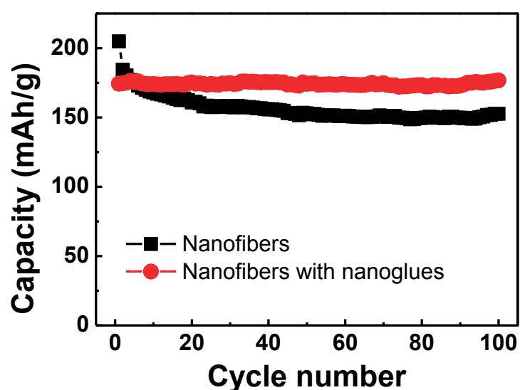
**Fig.S4** Cycle performance of  $\text{TiO}_2$  batteries.
