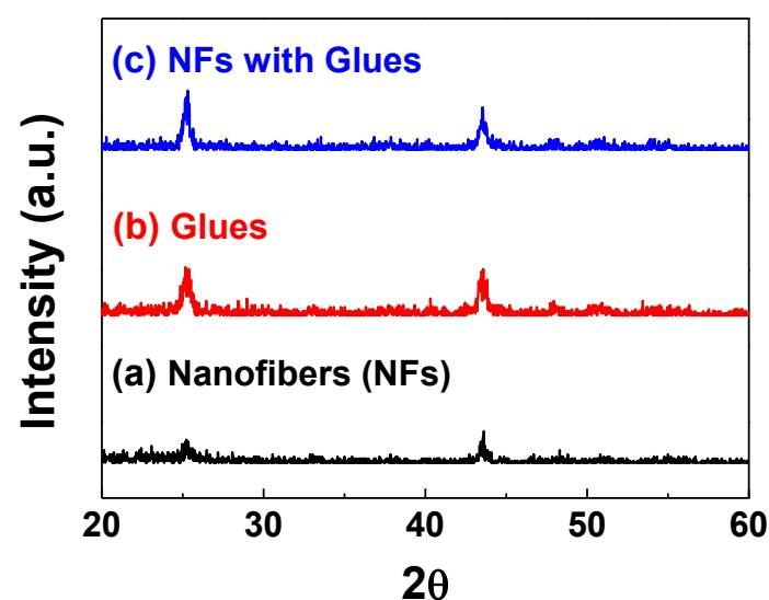
**Fig.S1** XRD patterns of  $\text{TiO}_2$  nanomaterials (a)  $\text{TiO}_2$  nanofibers, (b)  $\text{TiO}_2$  nanoglues, and (c)  $\text{TiO}_2$  nanofiber with nanoglues.
