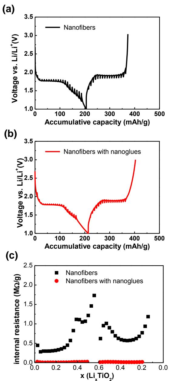
**Fig.S6** GITT voltage profiles of (a)  $\text{TiO}_2$  nanofibers electrode and (b)  $\text{TiO}_2$  nanofibers with nanogluces electrode, and (c) internal resistance of both electrodes.
