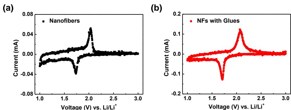
**Fig.S3** Cyclic voltammetry (CV) curves of (a)  $\text{TiO}_2$  nanofibers and (b)  $\text{TiO}_2$  nanofibers with nanoglues between 3.0 V and 1.0 V at a scan rate of  $0.2 \text{ mVs}^{-1}$ .
