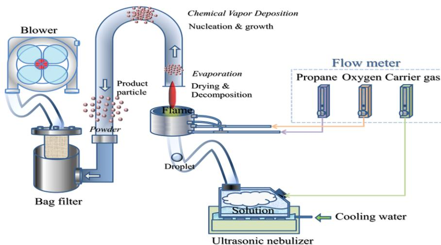
**Fig. S1.** Schematic diagram of the flame spray pyrolysis process.
