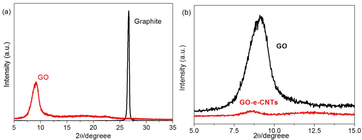
**Figure S4.** (a) XRD patterns of graphene oxide (GO) and graphite, (b) XRD patterns of GO and GO-e-CNTs. The weight ratio of GO and CNTs is 1:1.
