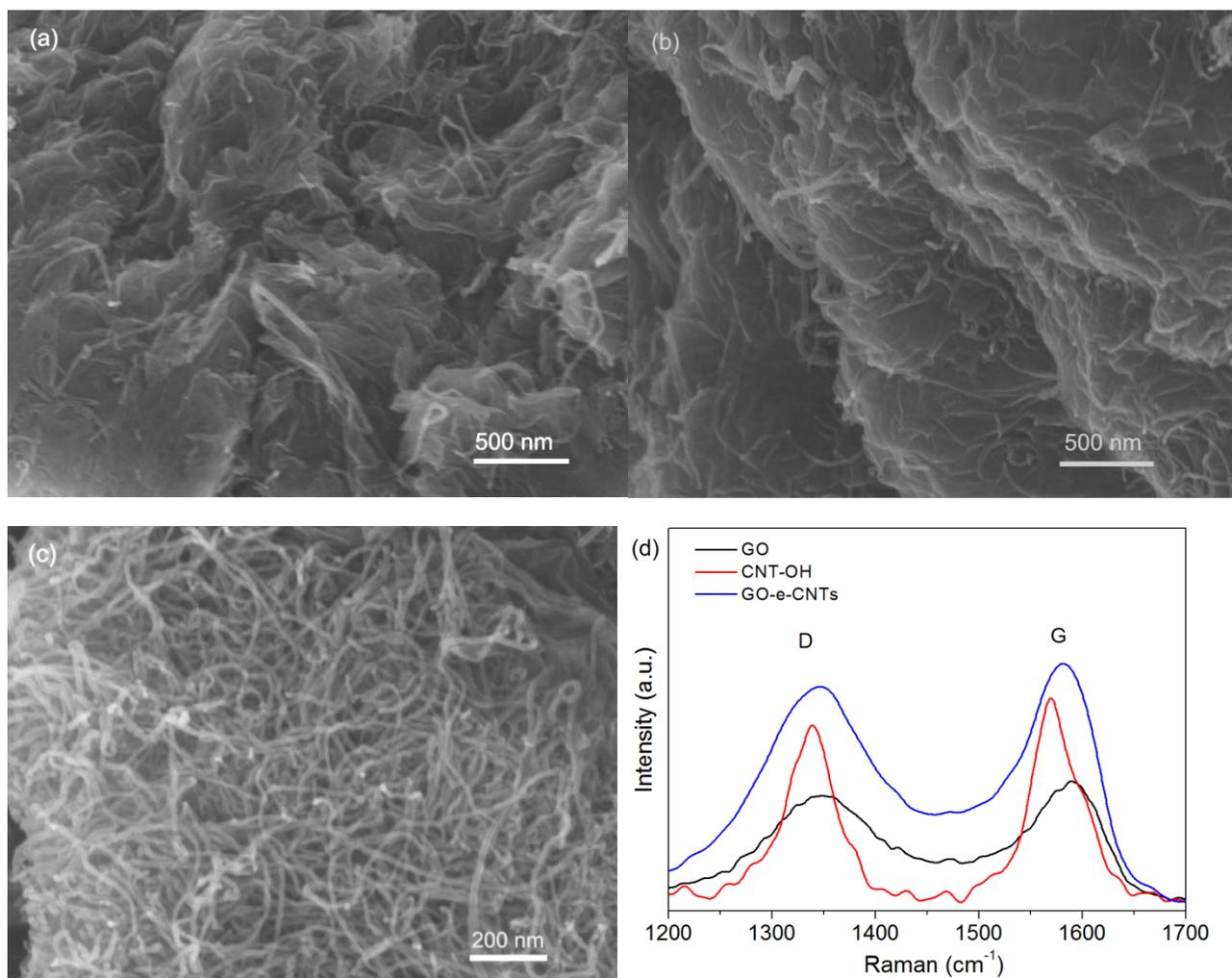
**Figure S3.** a,b) SEM images of in-site reduced GO-e-CNTs, clearly showing that the CNTs are encapsulated by the reduced GO sheets; Mass ratio of GO and CNT is 1 for GO-e-CNTs. c) SEM image of CNT-OH; d) Raman spectra of GO, CNT-OH and GO-e-CNTs.
