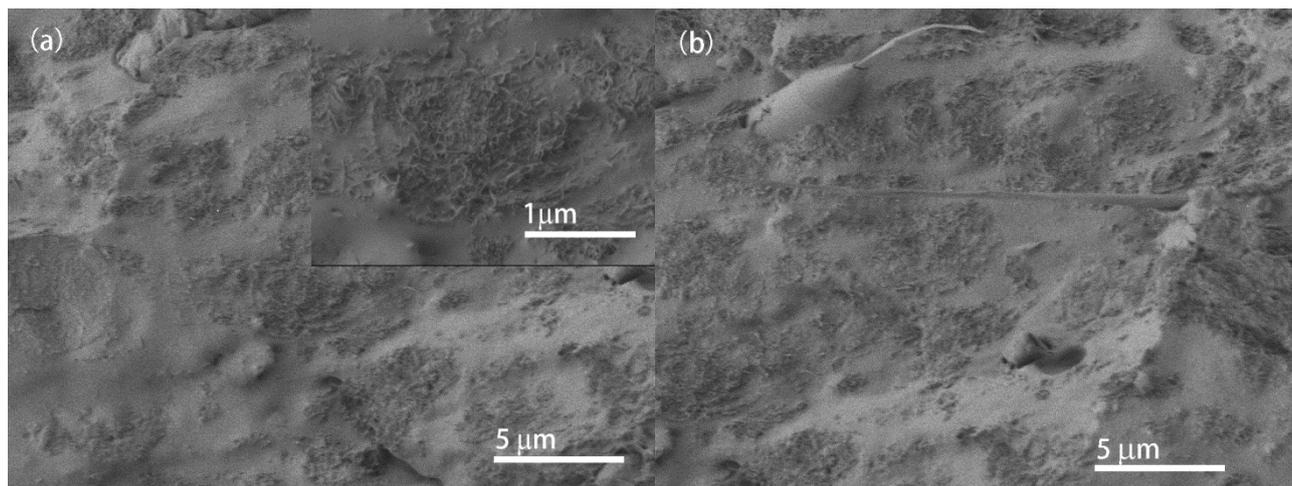
**Figure S5.** Representative SEM images of the CNT composites with a) 15 wt% and b) 20 wt% CNTs.
