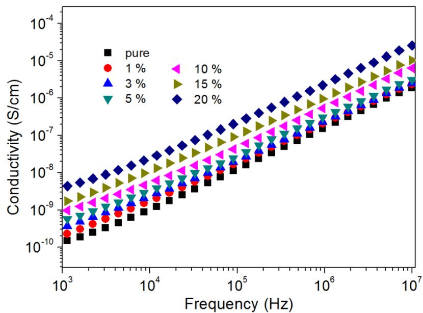
**Figure S8.** Frequency-dependent electrical conductivity of the GO-e-CNT composites with various loadings of CNT from  $10^3$  to  $10^7$  Hz.
