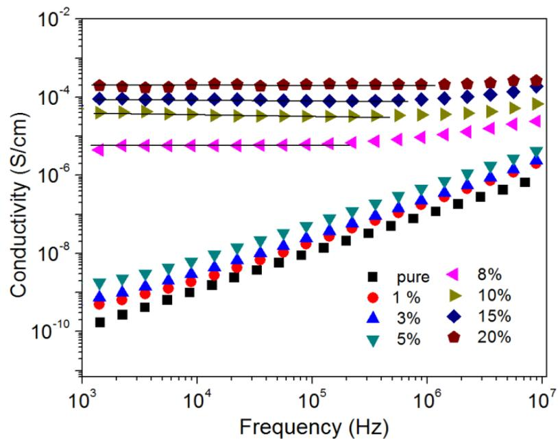
**Figure S6.** Frequency-dependent electrical conductivity of the pristine CNT composites with various loadings of CNTs.
