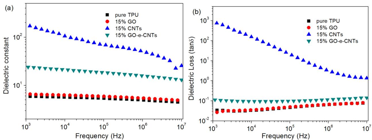
**Figure S7.** Frequency-dependent dielectric constant (a) and dielectric loss tangent (b) of the composites with CNT, GO, and GO-e-CNTs.
