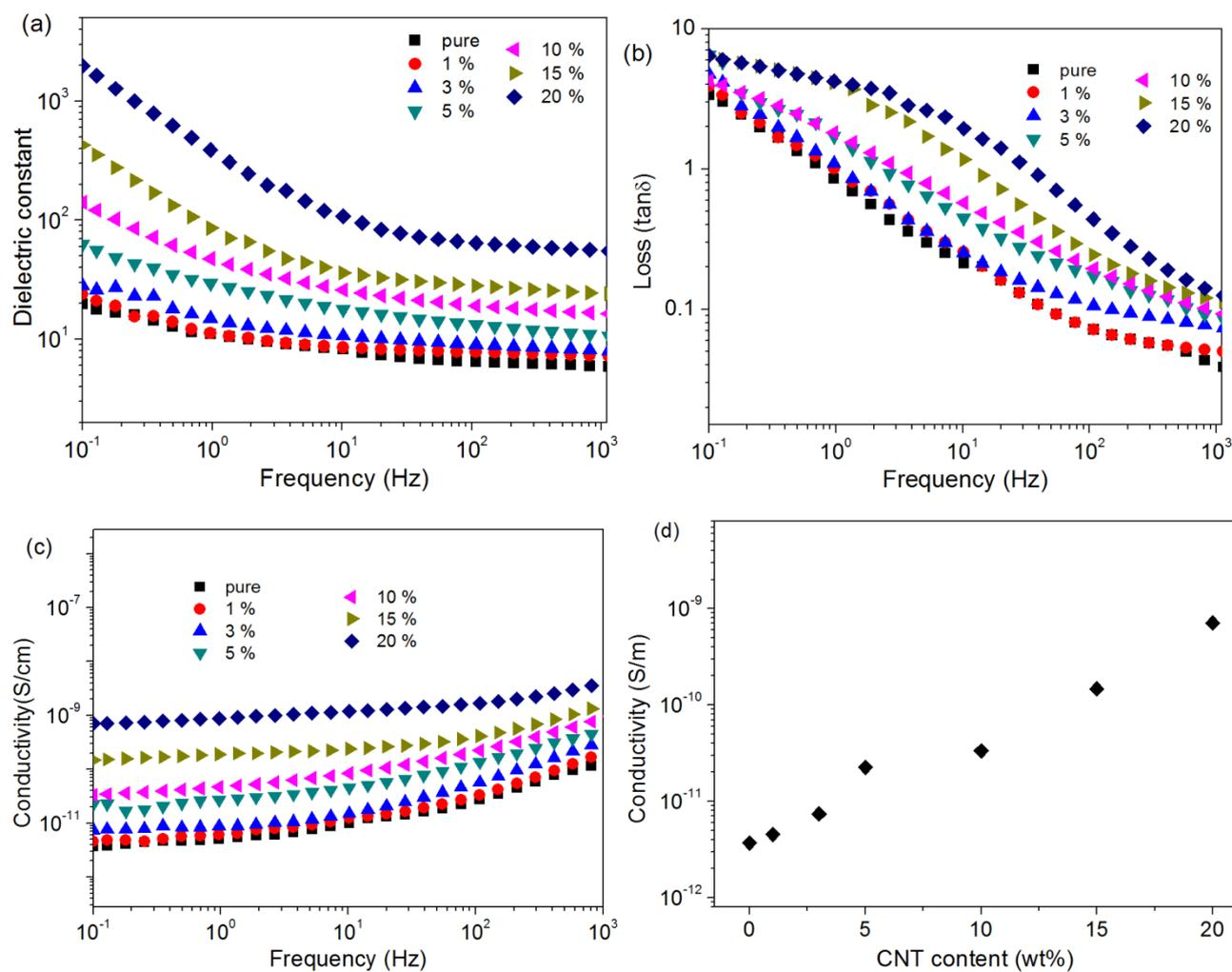
**Figure S9.** Frequency-dependent dielectric constant (a), dielectric loss tangent (b) and conductivity (c) of the composites as a function of the GO-e-CNT loading from 0.1 to  $10^3$  Hz; (d) Variation of electrical conductivity (b) of the GO-e-CNT/PU composite films as a function of the mass fraction of CNTs at 0.1 Hz.
