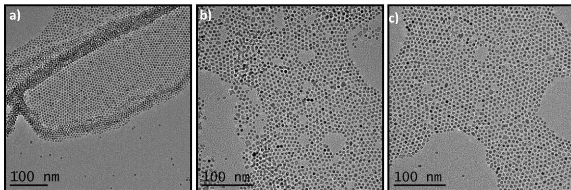
**Figure S.5:** Single layer assemblies of  $\text{ZrO}_2$  nanocrystals using the colloidal solutions with different solvents. a) Chloroform; b) Toluene; c) Hexane.
