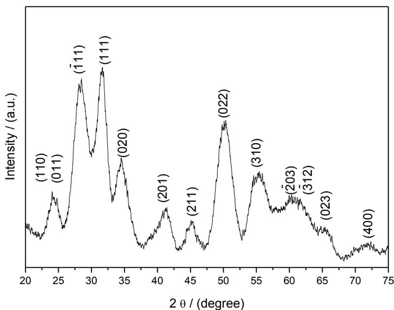
**Figure S.3:** X-ray diffraction for the ZrO<sub>2</sub> synthesized in oleic acid.
