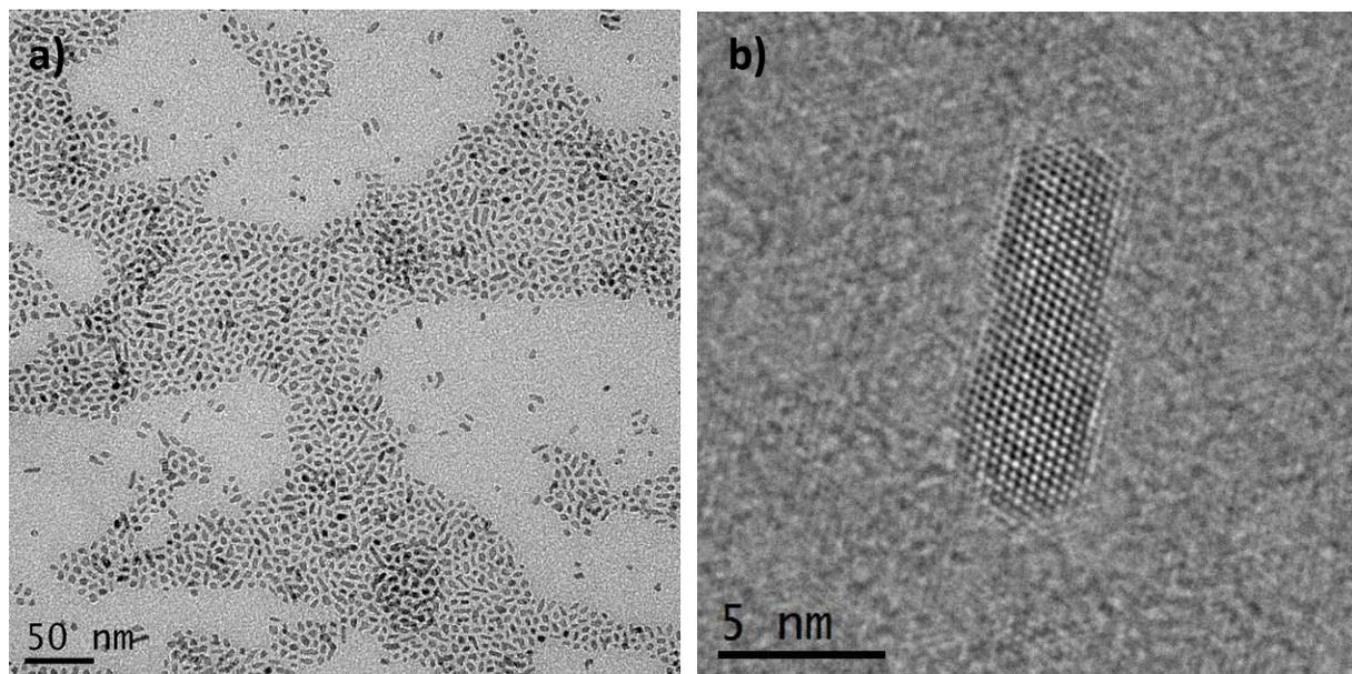
**Figure S.4:** TEM image for the ZrO<sub>2</sub> synthesized in OA. a) low magnification image for general visualization. b) HRTEM image of one ZrO<sub>2</sub> NC obtained in oleic acid.
