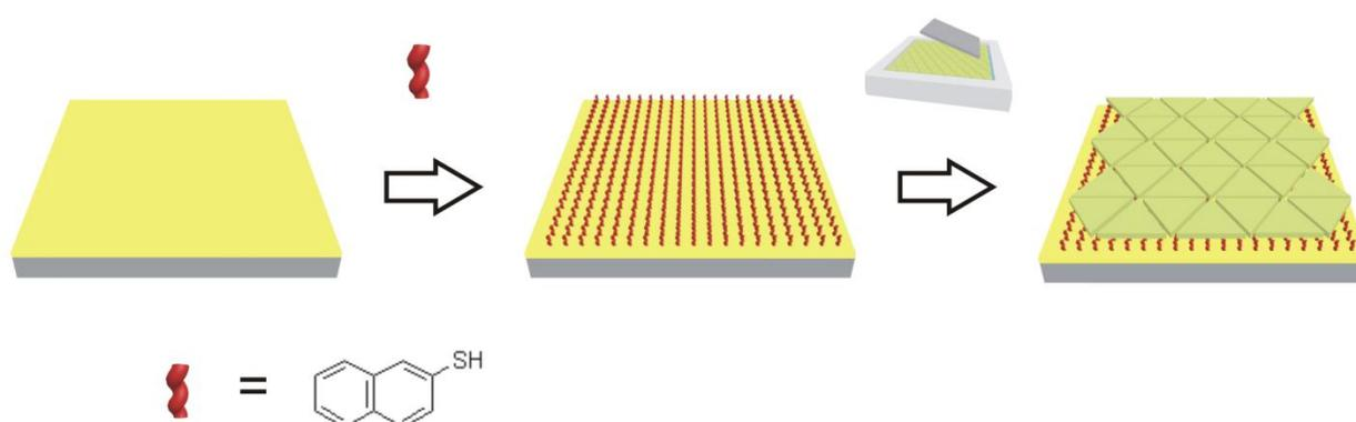
**Fig. S1** Schematic illustration of SERS substrates preparation for the (a) monolayer-over-dielectric and (b) monolayer-over-mirror layouts. In (a), film transfer of Au prism monolayers onto Si substrate was carried out, followed by functionalizing with the respective thiol molecules. In (b), the Au coated substrates were first functionalized with the probe molecules before the film transfer.
