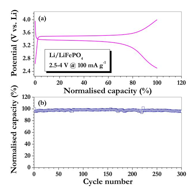
**Figure S5:** (a) Normalized charge-discharge curves of Li/LiFePO<sub>4</sub> cells cycled between 2.5-4 V at current density of 100 mA g<sup>-1</sup> in room temperature, and (b) cycling performance of charge/discharge capacity *vs.* cycle number.
