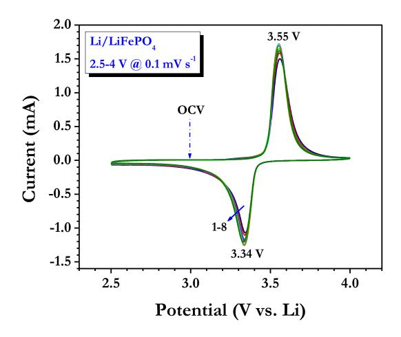
**Figure S4**. Cyclic voltammogram of Li/LiFePO<sub>4</sub> cells cycled between 2.5-4 V at scan rate of 0.1 mV  $\rm s^{-1}$ .
