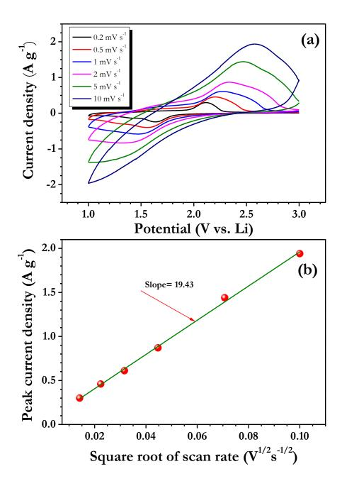
**Figure S3**. (a) CV traces of Li/electrospun TiO<sub>2</sub> hollow fibers cells recorded at various scan rates between 1-3 V vs. Li in ambient temperature conditions and (b) Relationship between the peak current density and the square root of scan rate in anodic processes.
