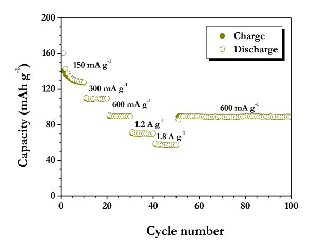
**Figure S1.** Galvanostatic cycling profiles of TiO<sub>2</sub> hollow nanofibers in half-cell configuration between 1-3 V vs. Li at various current densities in ambient temperature conditions. Plot of capacity vs. cycle number.
