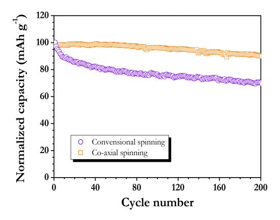
**Figure S2**. Galvanostatic cycling profiles of electrospun anatase nanofibers prepared through two different electrospinning techniques such as conventional single needle procedure and coaxial electrospinning technique.
