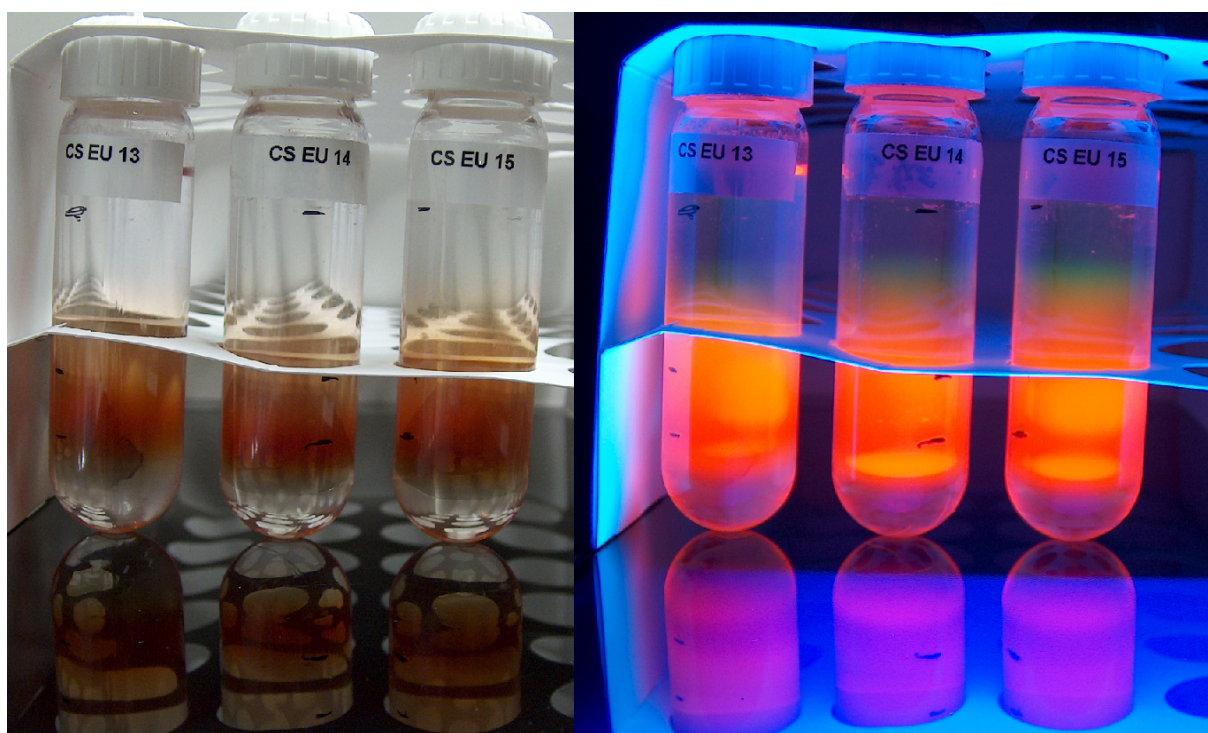
Figure S2: Images of PI- b -PEG encapsulated QDs after sucrose gradient centrifugation with (right) and without (left) UV irradiation.
