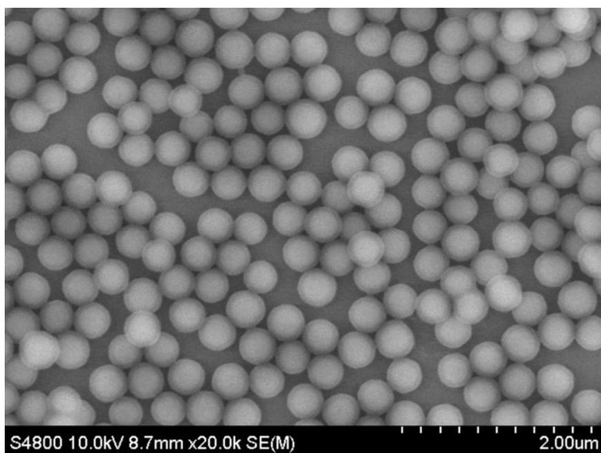
**Fig. S1** SEM image of SiO<sub>2</sub>@RF core-shell spheres
