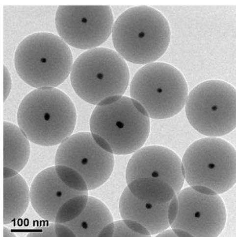
**Fig. S9** TEM image of Au@SiO<sub>2</sub>.
