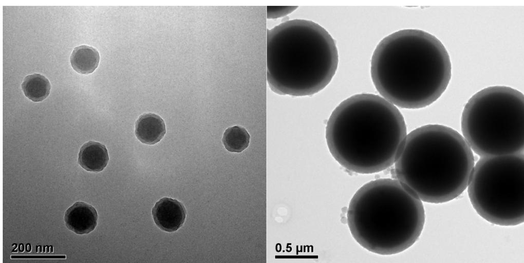
**Fig. S3** TEM images of SiO<sub>2</sub>@RF core-shell spheres with different diameter of SiO<sub>2</sub> cores: (a) 100 nm and (b) 750 nm.
