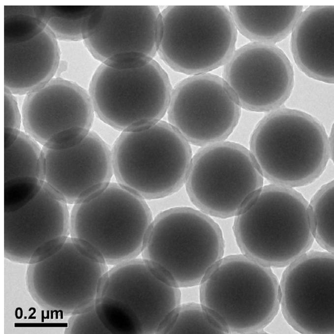
**Fig. S2** TEM image of SiO<sub>2</sub>@RF core-shell spheres obtained by replacing CTAB with CTAC.
