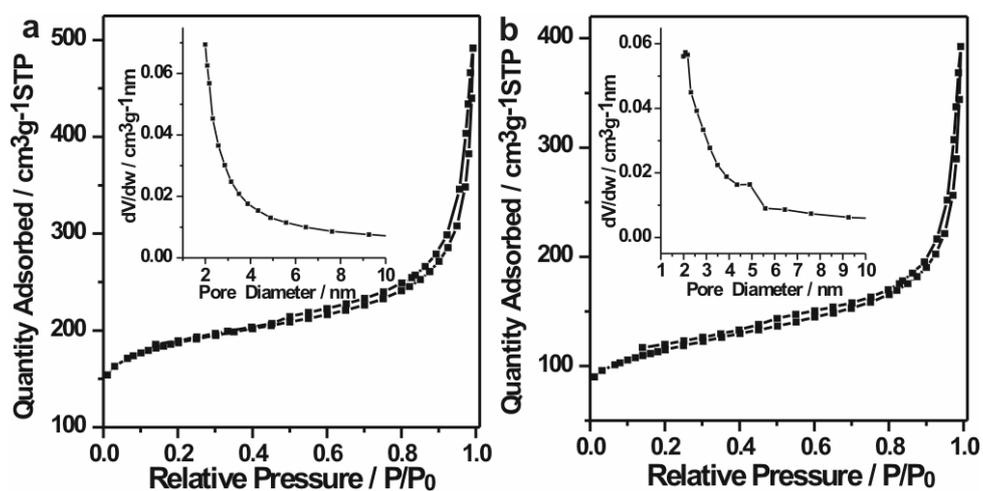
**Fig. S5**  $N_2$  sorption isotherms of HCS-260 (a) and HGS-260 (b), inset: the pore size distribution.
