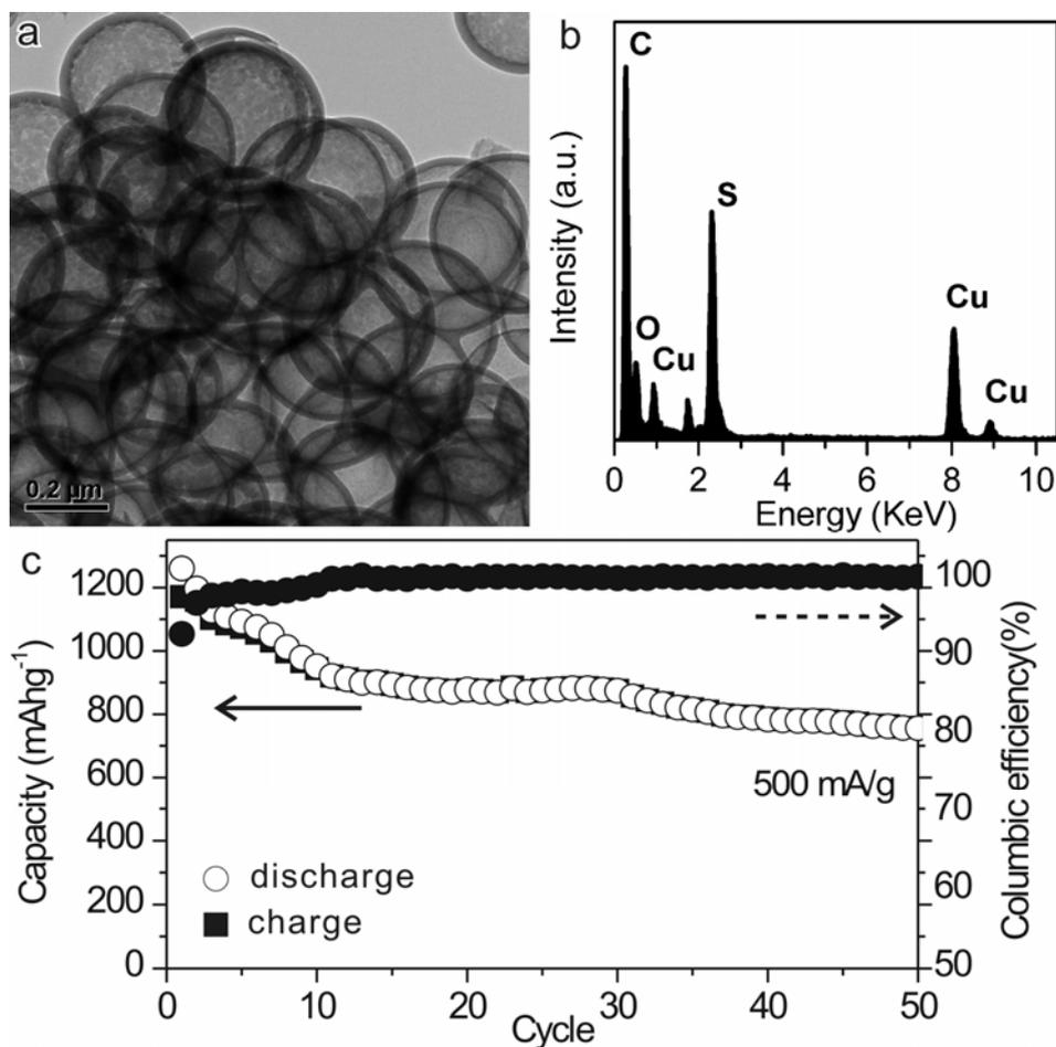
**Fig. S6** TEM image (a) and EDX spectrum (b) of HCS-260/sulfur composites, (c) cycling performance of lithium-sulfur batteries with HCS-260/sulfur cathode.
