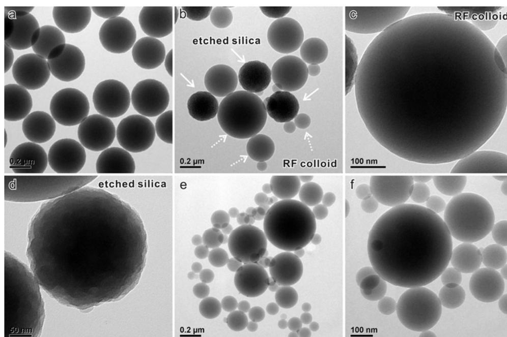
**Fig. S4** TEM images: (a) SiO<sub>2</sub> spheres, (b) etched SiO<sub>2</sub> spheres and RF colloids obtained by hydrothermal reaction of phenol and hexamethylenetetramine in the presence of SiO<sub>2</sub> spheres, (c) typical RF colloid, (d) typical etched silica sphere, (e) and (f) etched SiO<sub>2</sub> spheres and RF colloids treated by HF aqueous solution.
