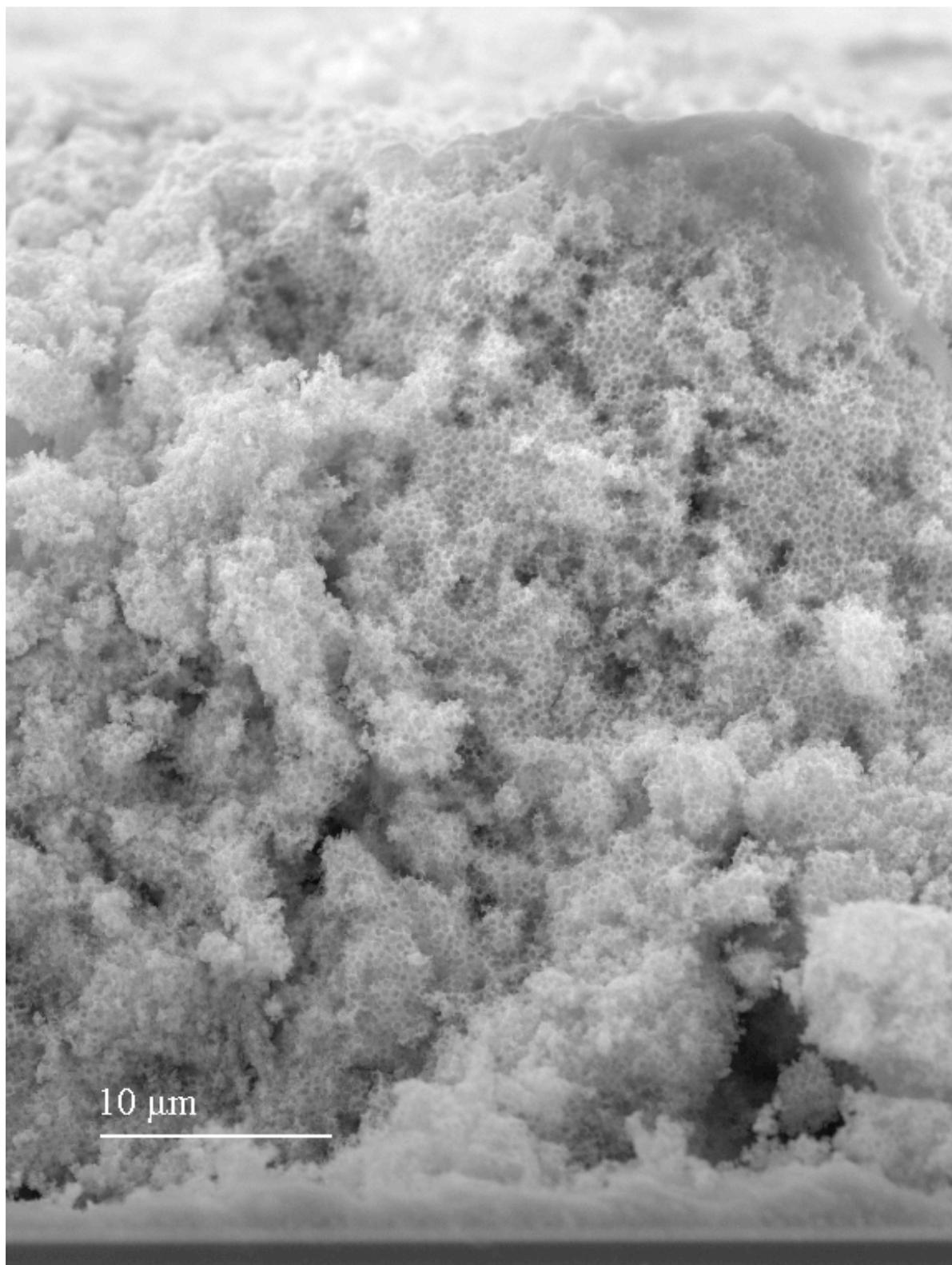
**Fig. S3** Cross-sectional SEM picture of a high-quality 3-D nanoporous FTO film as thick as 50 $\mu\text{m}$  on the FTO glass, indicating the uniform and interconnecting 3-D nanoporous structure.
