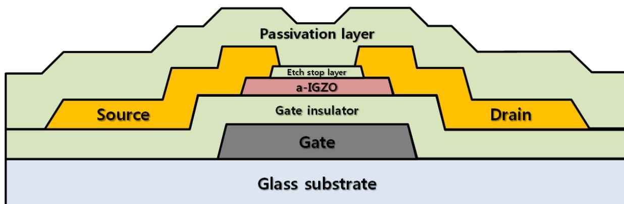
**Fig. S3** The device structure of a-IGZO TFT was an inverted-stagger type with a width-to-length (W/L) ratio of 100/10  $\mu\text{m}$  using a bottom gate.
