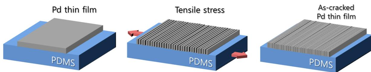
**Fig. S1** Fabrication of nano cracks in Pd TF. The Pd/PDMS substrate was mounted onto a stretching machine and nano cracks were created under a tensile stress
