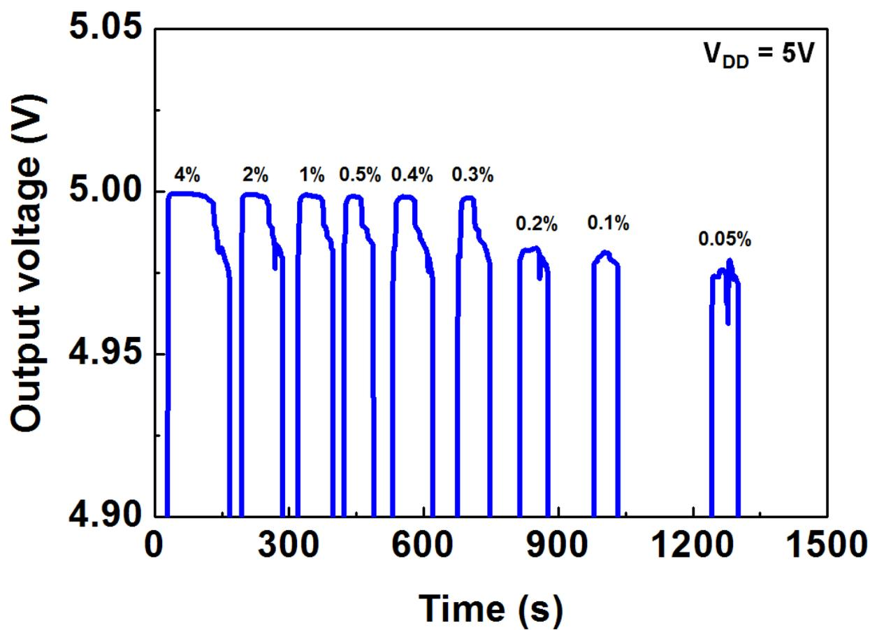
**Fig. S4** The magnified time domain  $V_{OUT}$  plot of Fig. 4b. The  $V_{OUT}$  signal from 0.05 % is 4.95 V which is only slightly lower than that (5.0 V) of 4 %  $H_2$  ambient.
