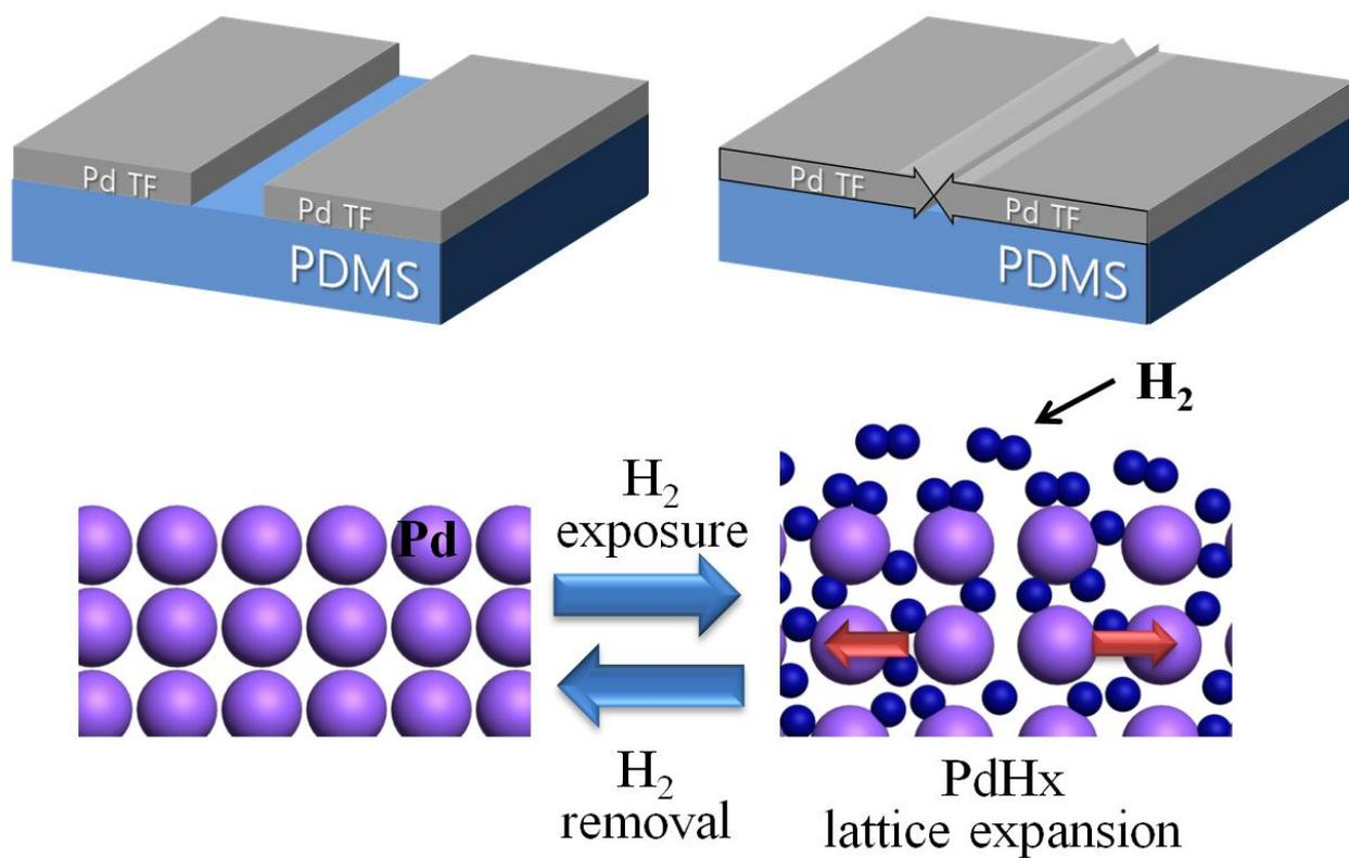
**Fig. S2** Illustration of physical contact in the Pd nanogap. H<sub>2</sub> adsorption and penetration into the lattice of Pd induces the volume expansion of Pd TF with phase change to PdH<sub>x</sub>, so that physical contact forms within the gap.
