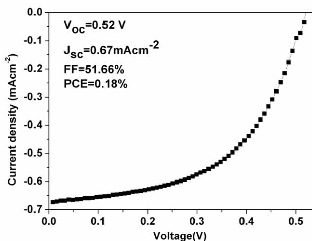
**Fig S1** Photocurrent density –voltage ( $J$ - $V$ ) characteristic of device with the photoanode of CuPc/TiO<sub>2</sub> under AM1.5 (100mWcm<sup>-2</sup>)
