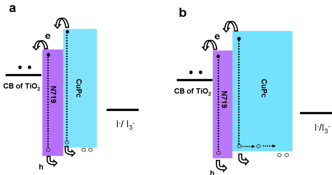
**Fig S4** Schematics of holes transfer process in DSSC with core-shell photoanode: a with thinner CuPc shell; b, with thicker CuPc shell.
