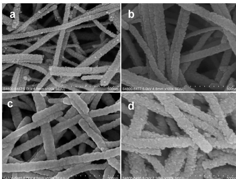
**Fig S3** SEM images of N719-sensitized  $TiO_2$  nanofibers coated with CuPc shell: a, without CuPc; b, 20nm CuPc; c, 30nm CuPc; d, 40nm CuPc
