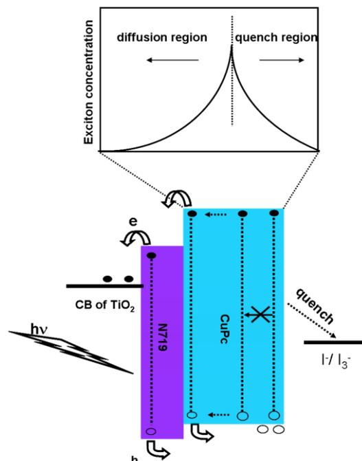
**Fig.S2** Schematic of electrolyte (I<sub>3</sub><sup>-</sup>) quenching the excited state of the CuPc and relationship between exciton concentration and distance from closer to N719 to far from N719
