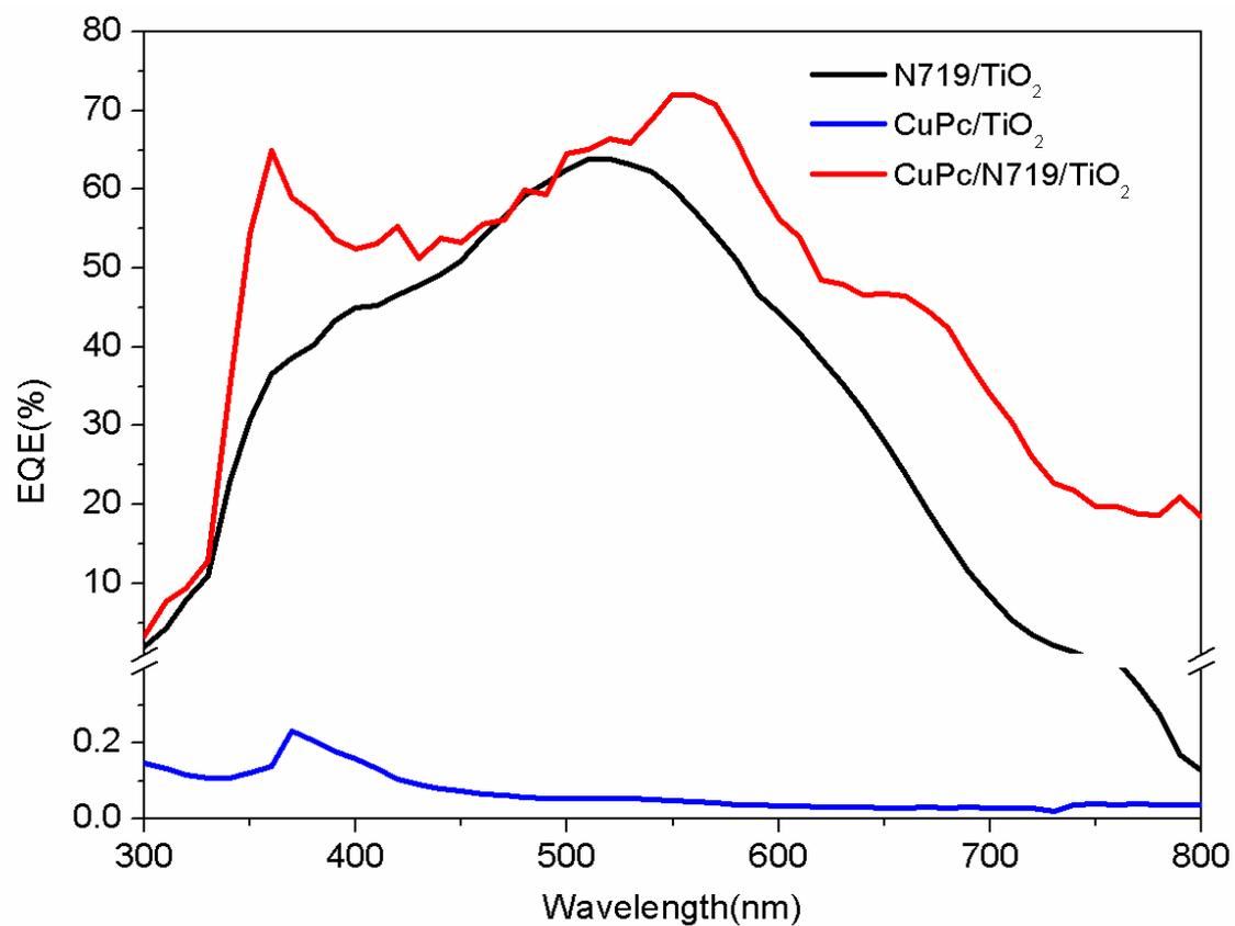
**FigS5** EQE versus wavelength of the DSSC with and without 30nm CuPc
