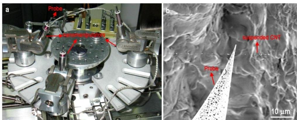
**Figure S5.** Nanomanipulator and probes fixed in a SEM. a) Nanomanipulator fixed in a SEM. b) A probe fixed on the nanomanipulators.
