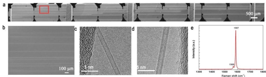
**Figure S1.** As-grown ultralong CNTs. a) and b): SEM images of as-grown CNTs with different magnifications. c) and d): TEM images of as-grown CNTs (double-wall CNTs and triple-wall CNTs). e) A typical Raman spectrum of as-grown CNTs.
