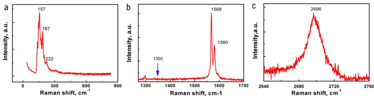
**Figure S3.** Raman spectra of a transferred CNT. (a) RBM-band. (b) D-band and G-band. (c) G'-band.
