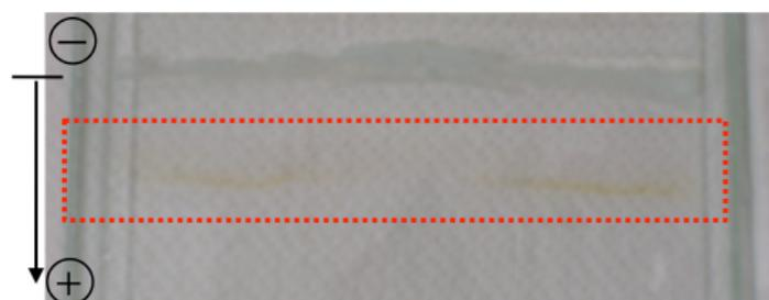
**Fig. S3.** Image of PAGE result for the synthesized  $\text{Au}_{25}(\text{SG})_{18}$ . Only a single band was observed.
