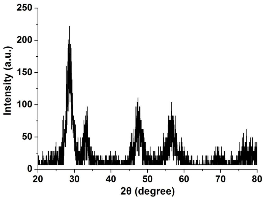
Figure S2. XRD pattern of CeO<sub>2</sub> mesoporous spheres.
