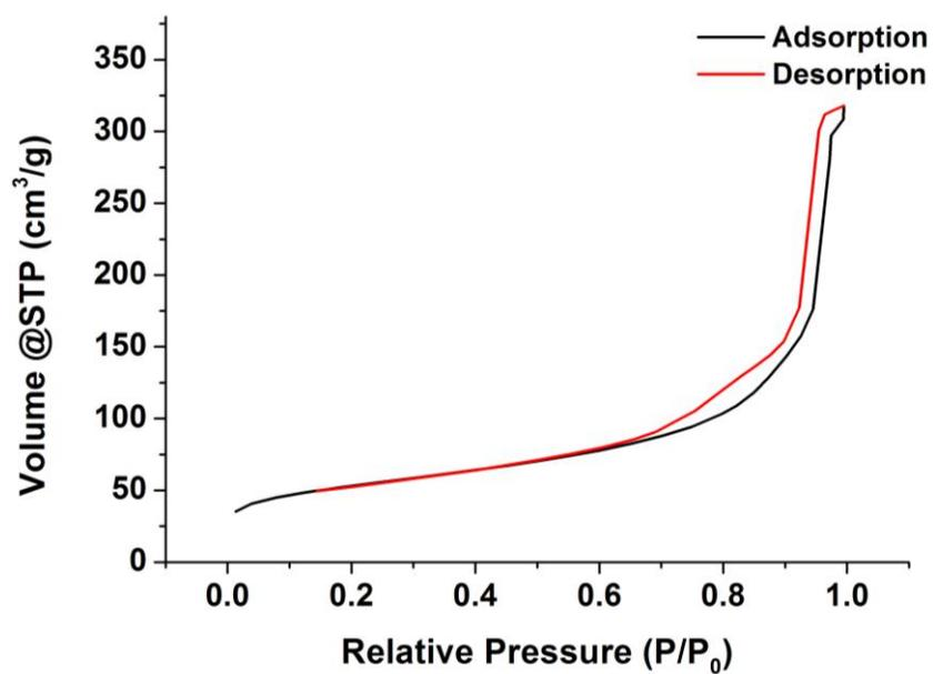
Figure S3. N<sub>2</sub> adsorption-desorption isotherm of Au@CeO<sub>2</sub>[P]
