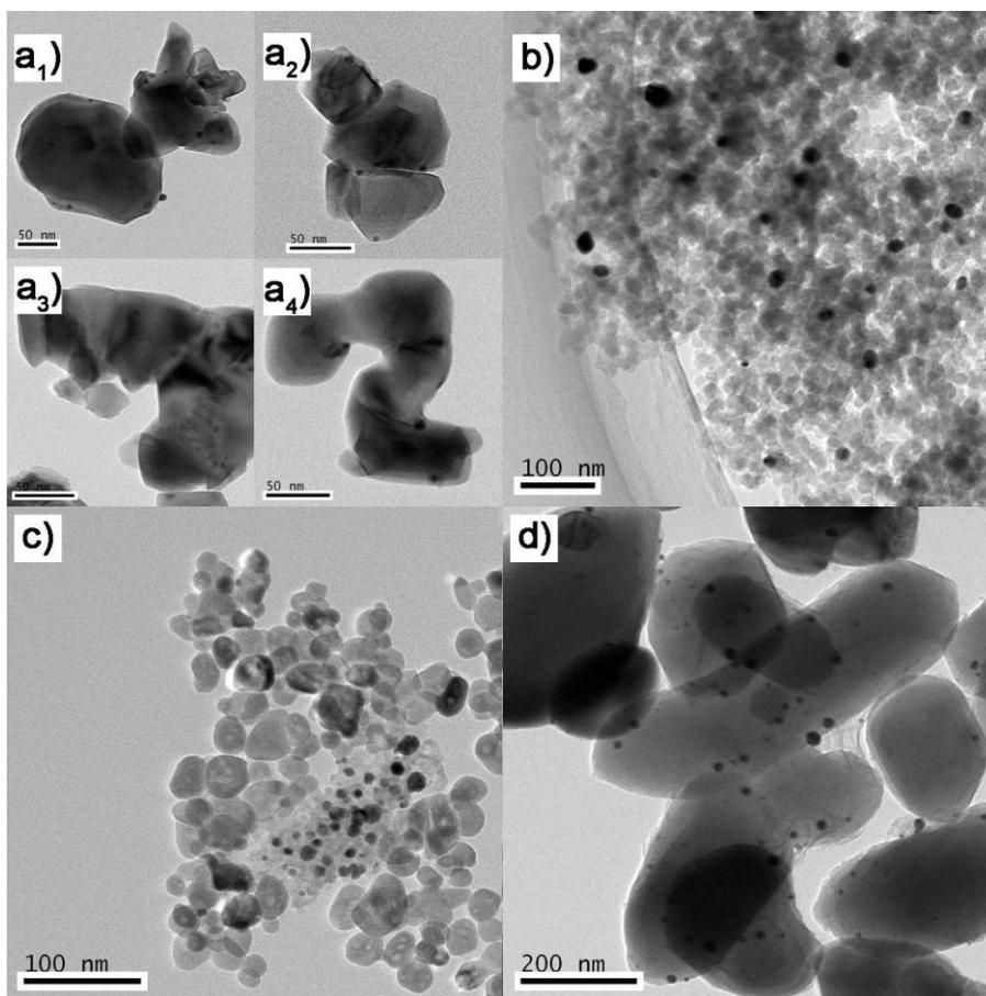
Figure S5. TEM images of Au NCs immobilized on different metal oxide supports (a: amorphous CeO<sub>2</sub>; b: SiO<sub>2</sub>; c: Fe<sub>2</sub>O<sub>3</sub>; d: TiO<sub>2</sub>. Scales in a, b, c, d are 50 nm, 100 nm, 100 nm and 200 nm, respectively).
