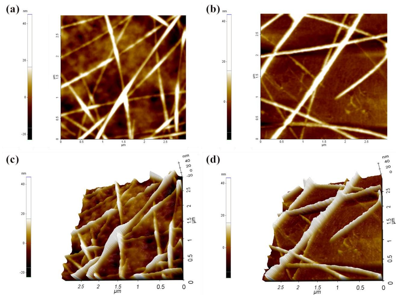
**Fig. S1** AFM topographies of AgNW and AgNW/Graphene TCEs on glass substrate: 2D images of (a) AgNW and (b) AgNW/Graphene TCEs, 3D images of (c) AgNW and (d) AgNW/Graphene TCEs.
