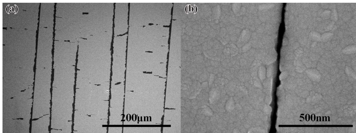
**Fig. S4** The SEM images of ITO/PEN TCE after mechanical flexibility test.
