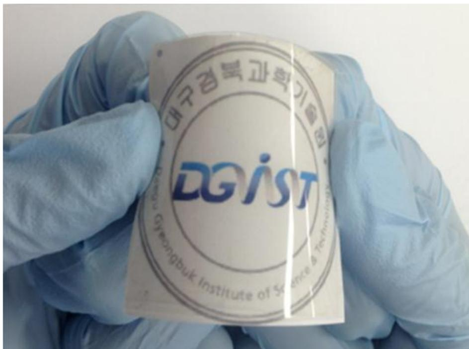
**Fig. S3** A photograph of flexible AgNW/Graphene/PEN TCE.
