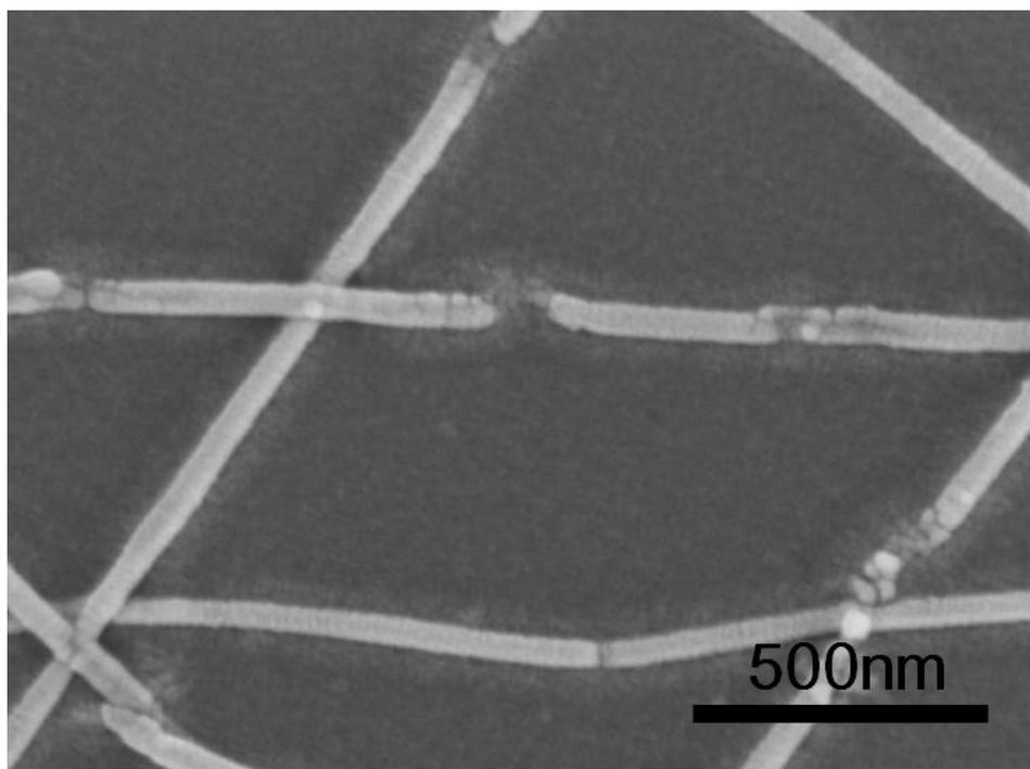
**Fig. S6** A SEM image of the AgNW TCE etched by acidic PEDOT:PSS solution.
