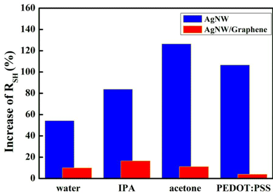
**Fig. S5** The chemical stability test of AgNW and AgNW/Graphene hybrid TCEs measured by dipping into various solvents.
