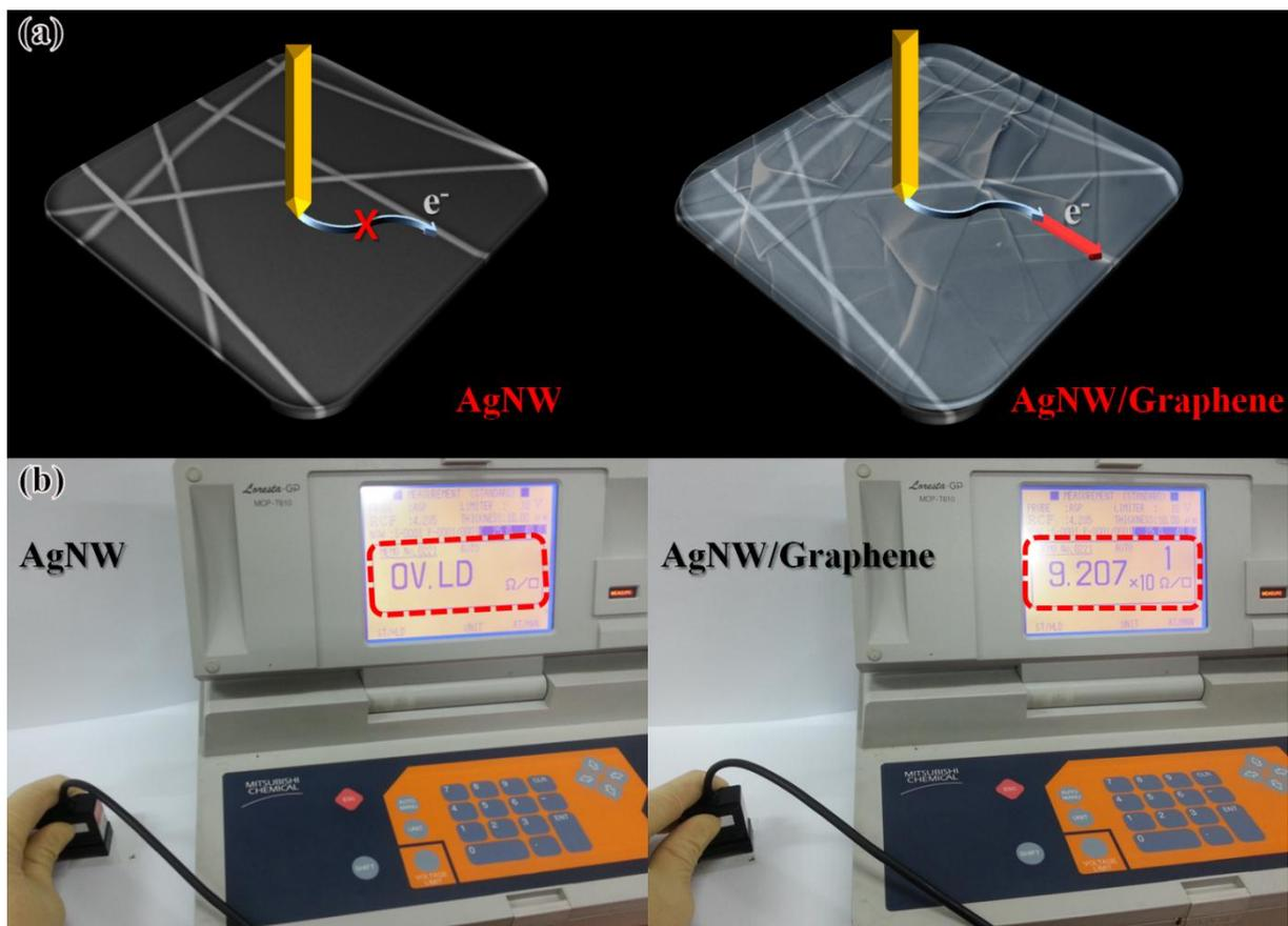
**Fig. S2** (a) Schematic illustration showing the roles of the graphene layer in improving the electrical connection between the AgNW TCE and conductive probe. (b) Images of electrical connection test of AgNW and AgNW/Graphene hybrid TCEs using a four-point probe measurement system.
