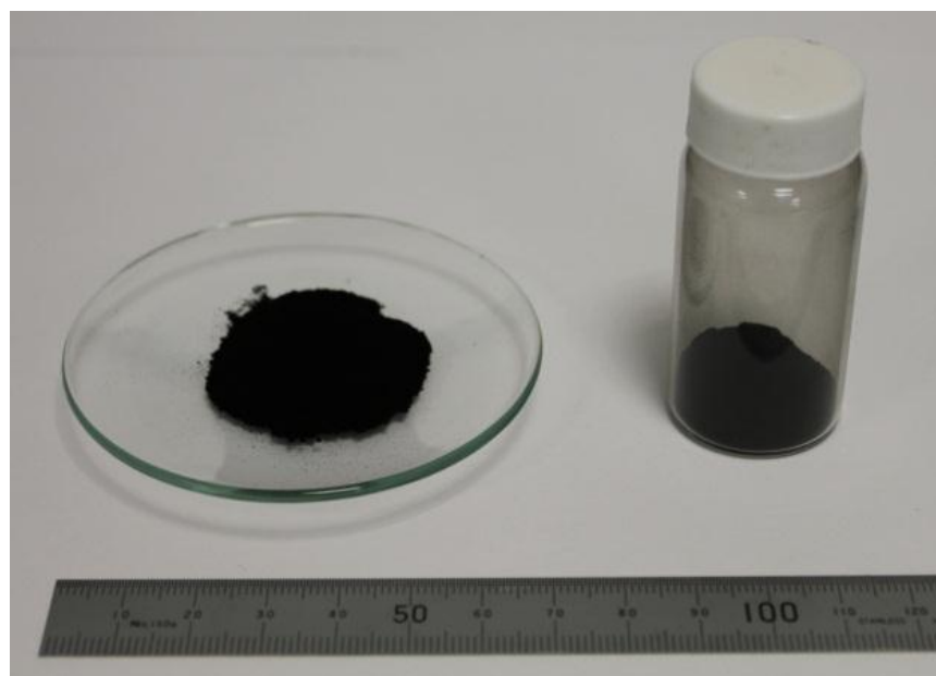
FigS1: Mass fabrication of ORR catalyst (unit of the ruler is millimeter).
