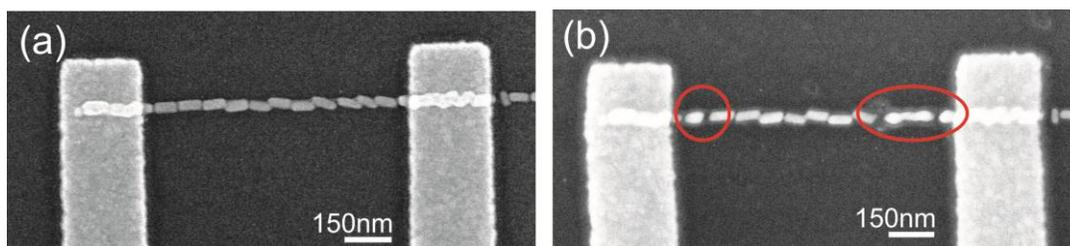
**Figure SI 4.** SEM picture of the topmost of the three Au NR chains in Figure 7a (a) prior to and (b) after electrical characterization. Some of the Au NRs within the chain apparently altered their shape after a voltage increase to 14 V, presumably as a consequence of Joule heating (red circles). In the middle chain and the lowermost chain no changes were visible, which indicates that most of the current passed through the topmost chain of Au NRs.
