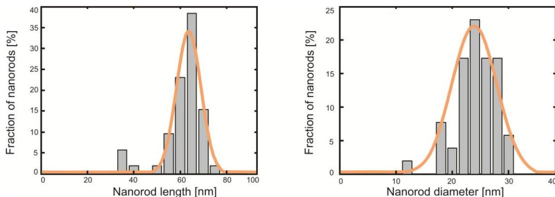
**Figure SI 1.** Size distribution of the Au NRs: by (a) length and (b) diameter.
