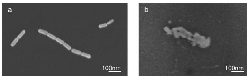
**Figure SI 2.** (a) Au NRs aligned into a line shifted during the removal of the underlying PMMA. (b) Au NRs fused due to the exposure to the O<sub>2</sub> plasma.
