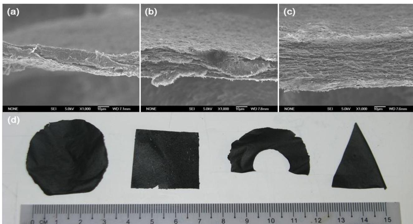
**Fig. S3.** SEM images (a-c) and digital picture (d) of RGO-PPy membranes with various thicknesses and shapes.
