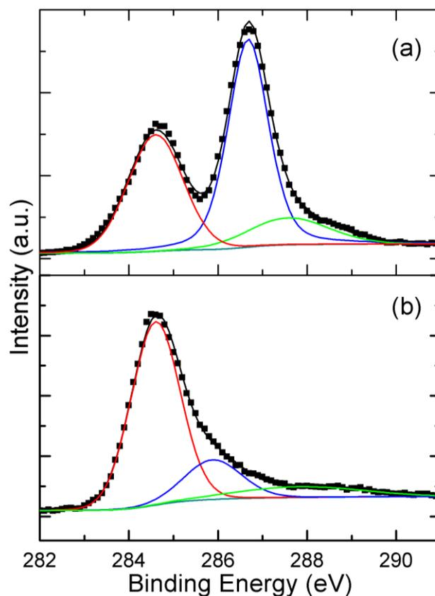
**Fig. S2.** Core level C 1s XPS spectra of GO (a) and RGO-PPy membrane (b).
