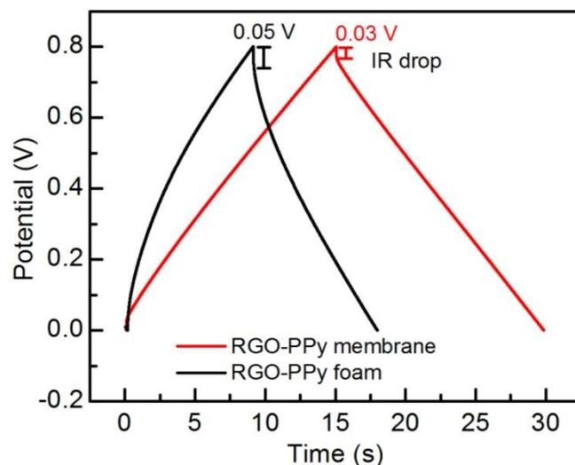
**Fig. S5.** Charge–discharge curves of two-electrode cells with symmetric RGO–PPy foam and RGO-PPy membrane, respectively. The IR drops for charge–discharge curves are shown in the Figure.
