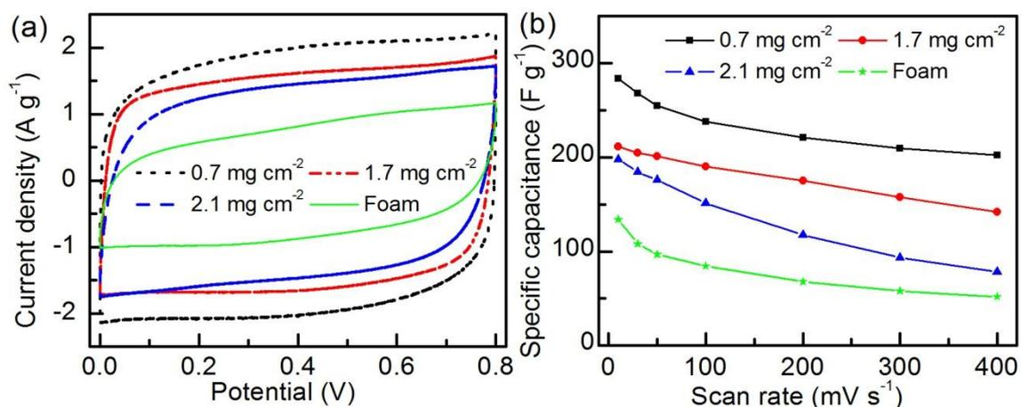
**Fig. S6.** Cycle voltammetric curves (a) and specific capacitance (b) of two-electrode cells with symmetric RGO–PPy foam ( $\sim 1.7\ mg\ cm^{-2}$ ) and RGO-PPy membranes with different thicknesses.
