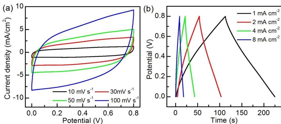
**Fig. S4.** Cycle voltammetry curves at various scan rates (a) and charge/discharge curves at various densities (b) of a two-electrode cell with RGO-PPy aerogel as both electrodes.
