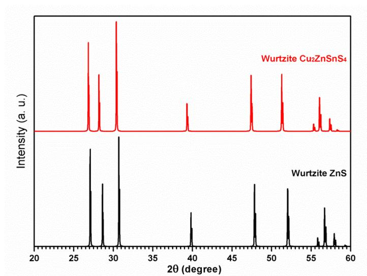
Figure S2. The XRD patterns of wurtzite ZnS and  $\text{Cu}_2\text{ZnSnS}_4$ . The XRD pattern of ZnS is obtained according to the JCPDS Card, No. 75-1534; and the XRD pattern of  $\text{Cu}_2\text{ZnSnS}_4$  is simulated by CrystalMaker and CrystalDiffract software.
