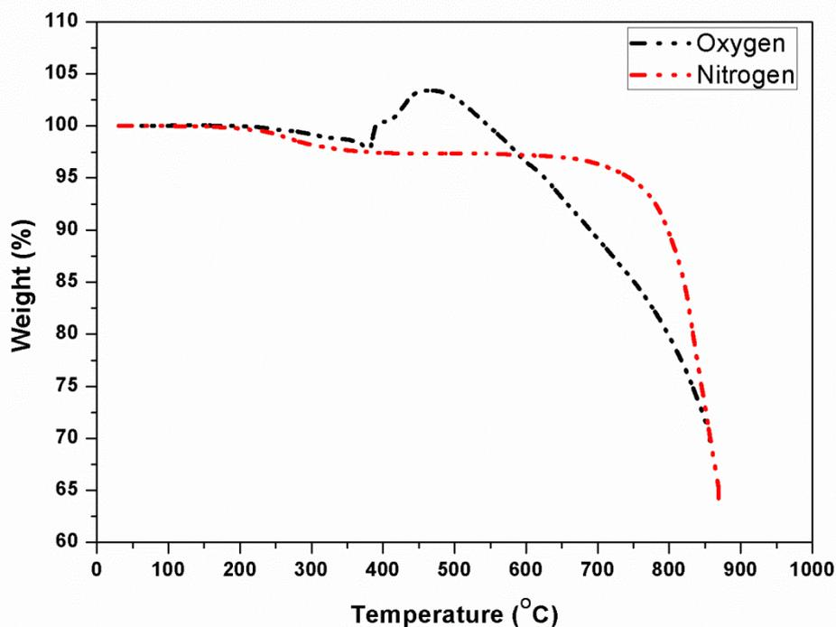
Figure S7. TGA curves of the as-synthesized CZTS nanoleaves. The first weight loss at about  $250^\circ\text{C}$  under oxygen flow is attributed to the loss of attached ligands, the weight gain is attributed to the oxidation during the oxygen circumstance. While, the weight loss at about  $250^\circ\text{C}$  under nitrogen flow is attributed to the loss of attached ligands,
