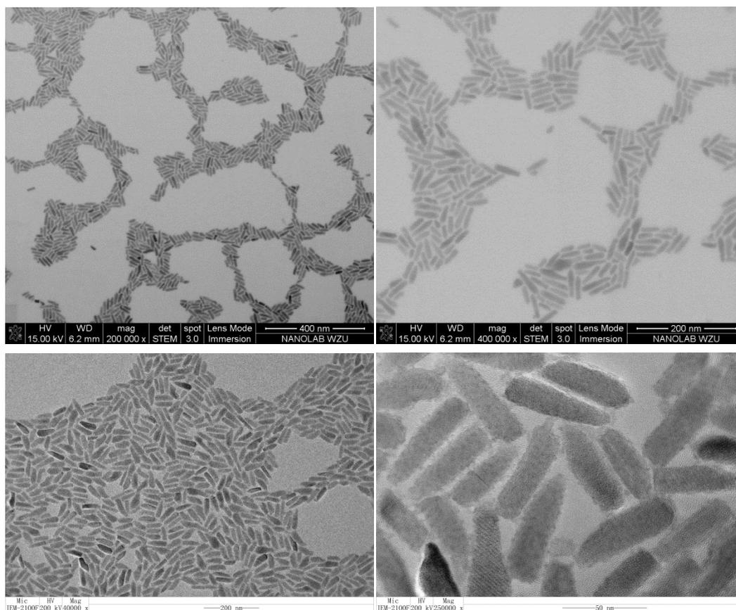
Figure S4. STEM and TEM images of  $\text{Cu}_2\text{ZnSnS}_4$  nanomaterials prepared at the presence of OLA, OA, and DT.
