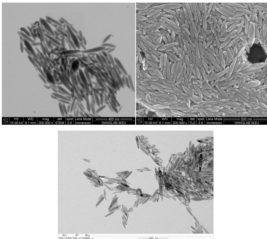
Figure S3. STEM and SEM images of  $\text{Cu}_2\text{ZnSnS}_4$  nanomaterials prepared at the presence of octadecene.
