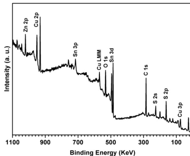
Figure S6. The survey spectrum of  $\text{Cu}_2\text{ZnSnS}_4$  nanoleaves.
