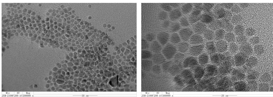
Figure S5. TEM images of  $\text{Cu}_2\text{ZnSnS}_4$  nanomaterials prepared at the presence of OLA and DT.
