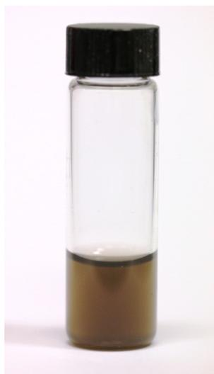
**Figure S2 : Water-based dispersion of NDs-H at 2 mg/ml.**
